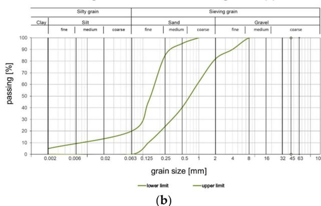
**Figure 3.** Grading curve corridors for the application as (a) an intensive green roof, according to FLL [50]; and (b) turfgrass, according to Austrian Standards B 2606-1 [38]; green lines indicate the upper and lower limit.
