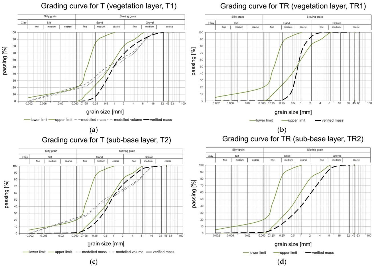
Figure 5. Grading curves of the tested engineered soils for turfgrass application in the vegetation layer (a,b) and the sub-base layer (c,d). (Horticultural reference soils (TR 1, TR 2) were not modeled).
