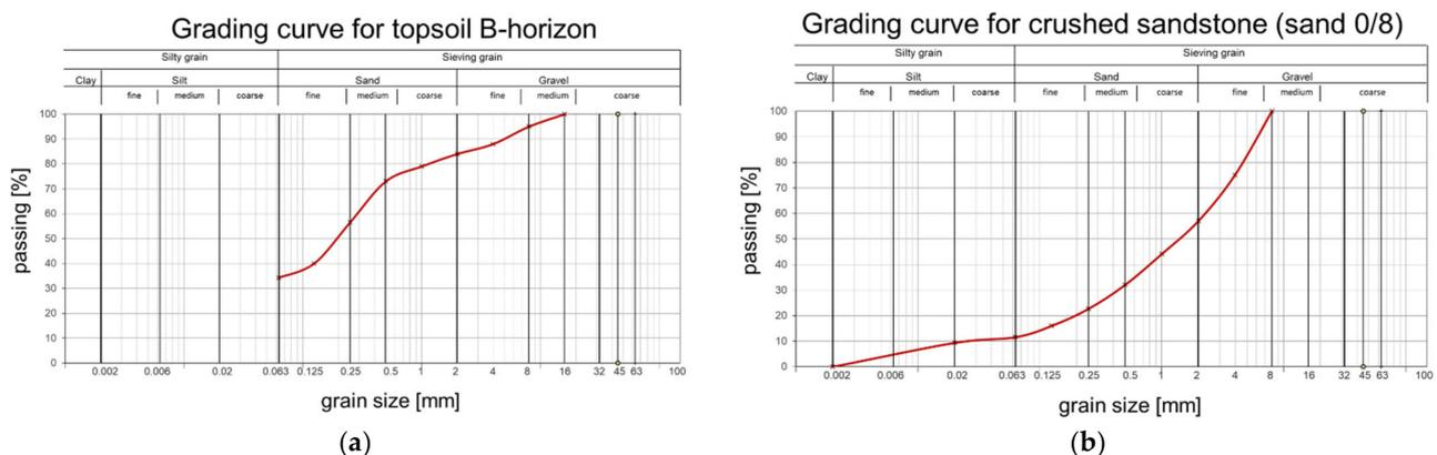
**Figure 2.** Grading curves of the excavated Wildgarten material: (a) topsoil B-horizon, (b) sandstone C-horizon (sand 0/8).
