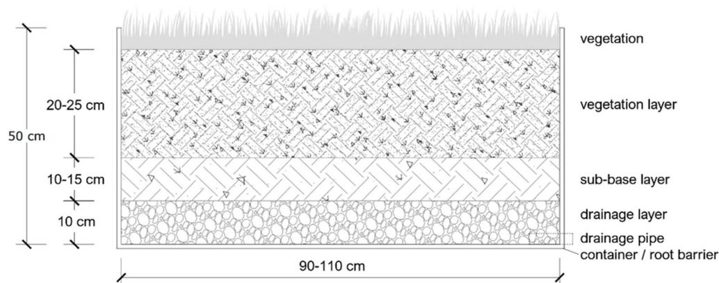
**Figure 1.** Applied standard profile of the mock-ups' setup for all tested applications.
