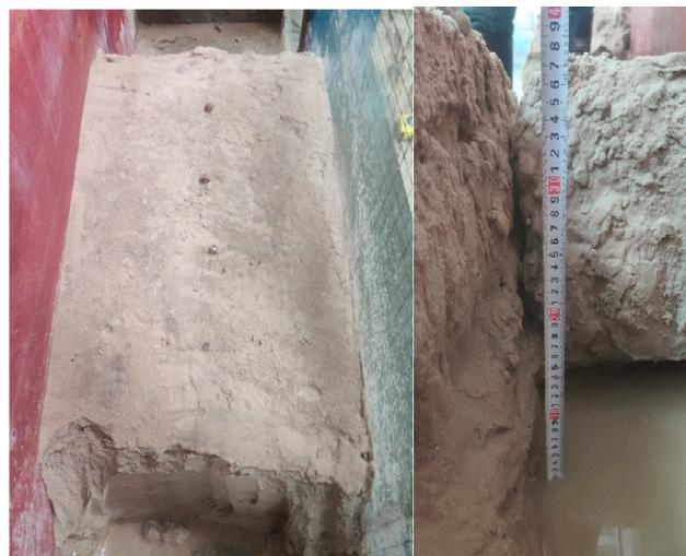
Figure 12. MICP-treated sand body (4-time MICP treatments).
