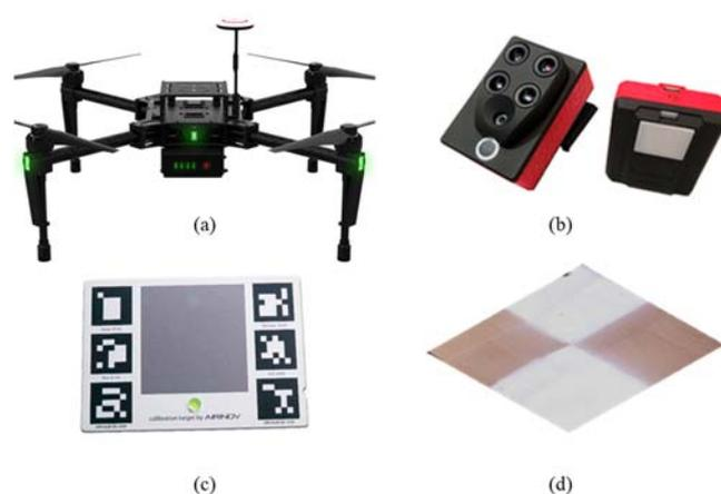
**Figure 2.** Equipment: (a) Matrice 100 quadcopter used for the survey; (b) Parrot Sequoia™ camera (image and irradiance sensors); (c) camera calibration target; (d) example of the control points.
