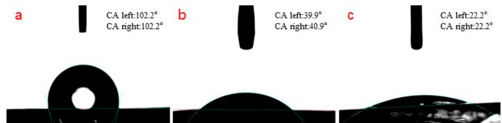
**Figure 7.** Contact angles between water, gasoline, and diesel and solid silicone: (a) water, (b) gasoline, (c) diesel.
