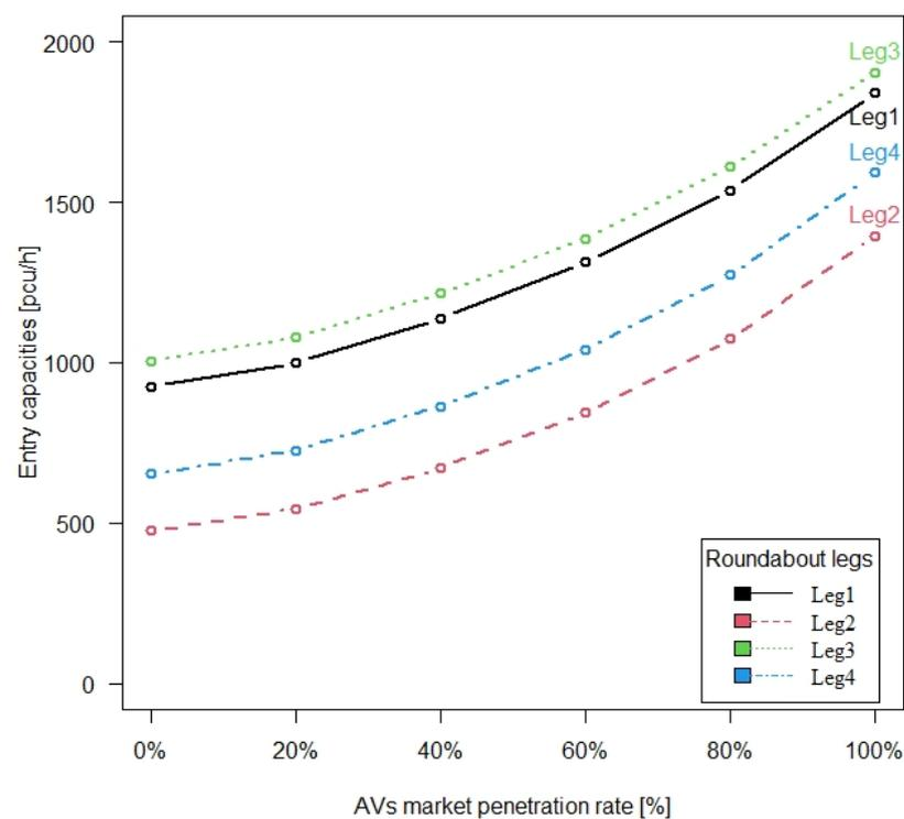
**Figure 4.** Entry capacities [pcu/h] by legs for different AV penetrations at 100% traffic flow level.
