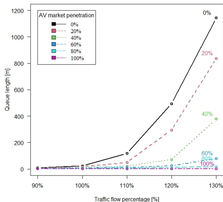
**Figure 5.** Queue length [m] on Leg1 with increasing flow at different AV penetration rates.
