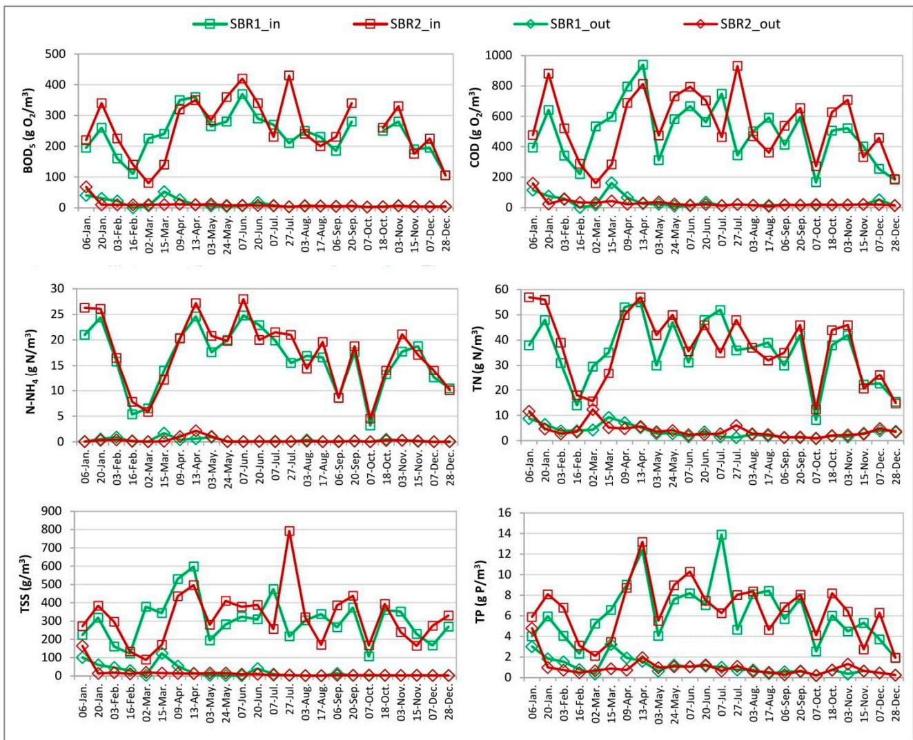
**Figure 8.** The course of the variability of wastewater treatment in SBR1 and SBR2 reactors.
