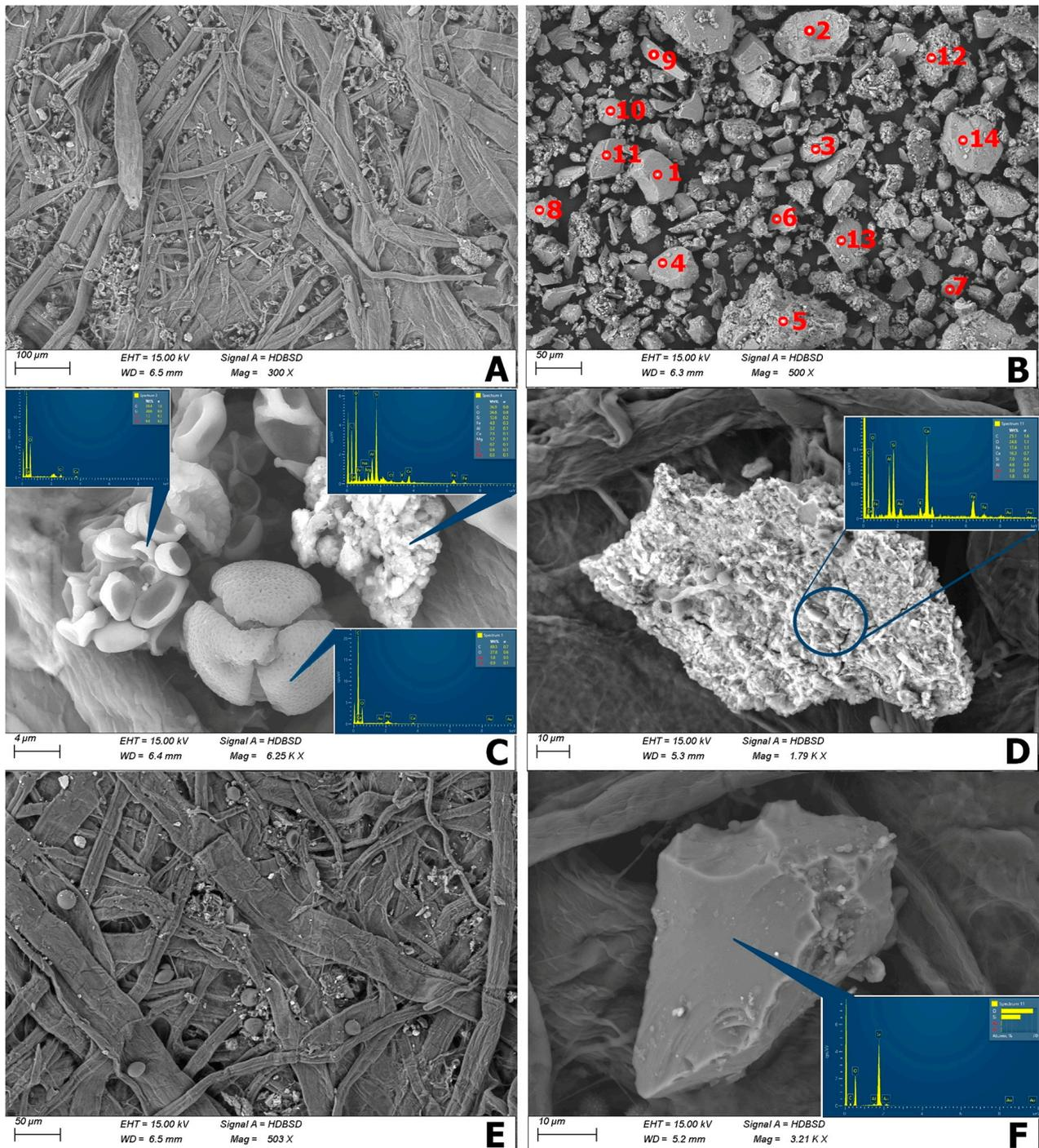
**Figure 5.** (A) Example of analysed area (undergrowth—zone 2); (B) PM collected from the side of the road, 1—orthoclase, 2—pyroxene, 3—calcium carbonate, 4—quartz, 5—plagioclase, 6—feldspar, 7,8—quartz, 9—pyroxene, 10—fly ash, 11—quartz, 12—amphibolite, 13—anorthoclase, 14—quartz; (C) example of observed particles; (D) asphalt particle; (E) sample trees—zone 4; (F) example of inorganic particle (quartz).
