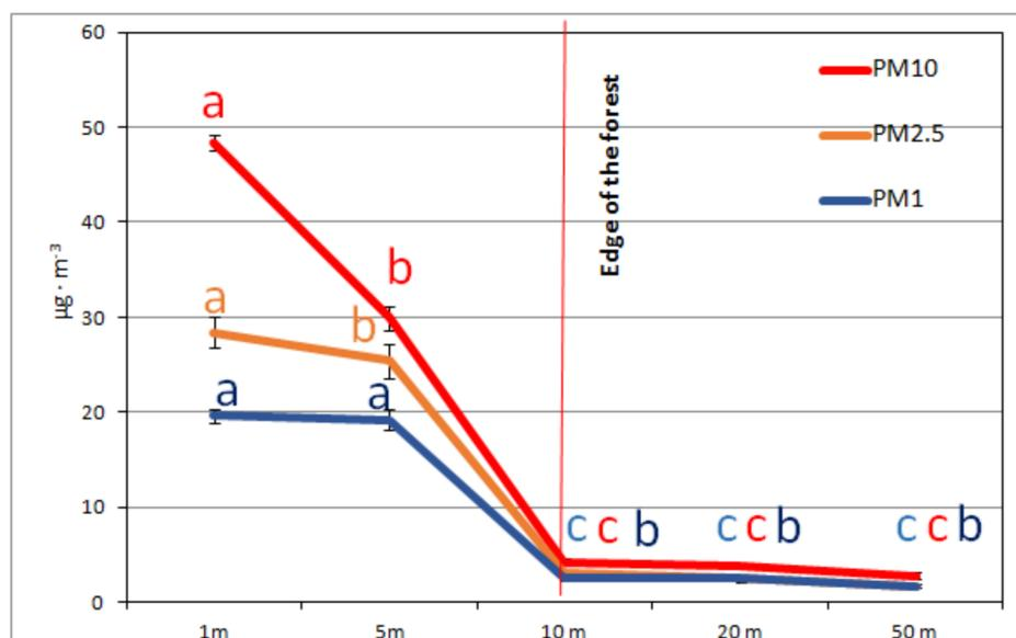
**Figure 3.** The concentration of PM<sub>10</sub>, PM<sub>2.5</sub>, and PM<sub>1</sub> in air depending on the distance from the source of pollution. Different letters in particular colours show statistically significant differences.
