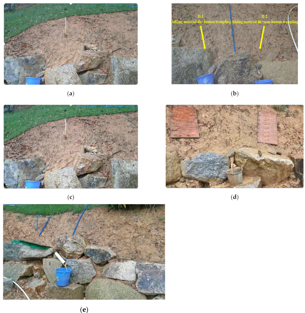
Figure 3. Field test of rainfall erosion in Zones I, II, III, IV, and V. (a) Natural soil; (b) added material for 4 h + manual trampling or non-manual trampling; (c) added materials for 12 h; (d) added materials for 24 h; (e) added materials for 48 h.
