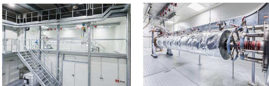
**Figure 4.** Pilot plant pulsation reactor (Kleinmengen-PR) at IBU-tec Advanced Materials AG, Weimar. View including the production hall (left) and a close-up view (right).
