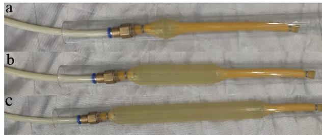
**Figure 3.** The inflating process of rubber airbag, (a) bubbles appear, (b) bubbles expand along the axial direction, (c) expansion complete.
