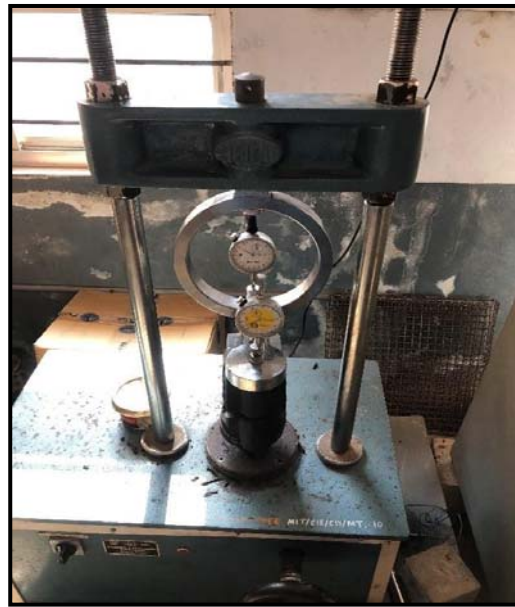
Figure 1. Marshall Stability and flow test setup.
