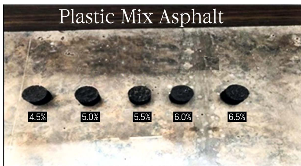
Figure 4. Tested specimen of plastic mix asphalt.
