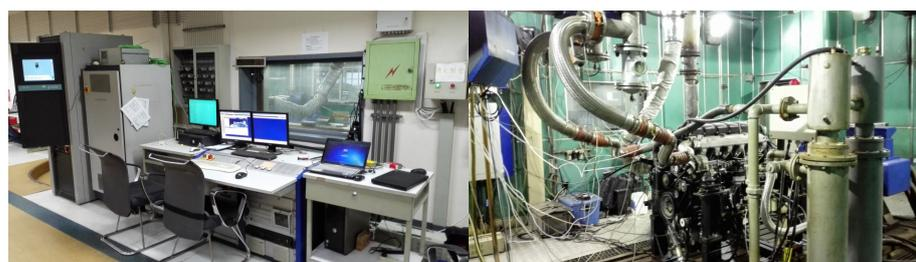
**Figure 5.** In-lab test: the test bench control platform (left) and the engine measurement system (right).
