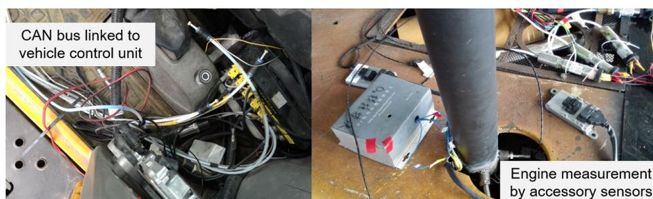
**Figure 4.** The vehicle data acquisition system and engine accessory sensors used in wheel loaders.
