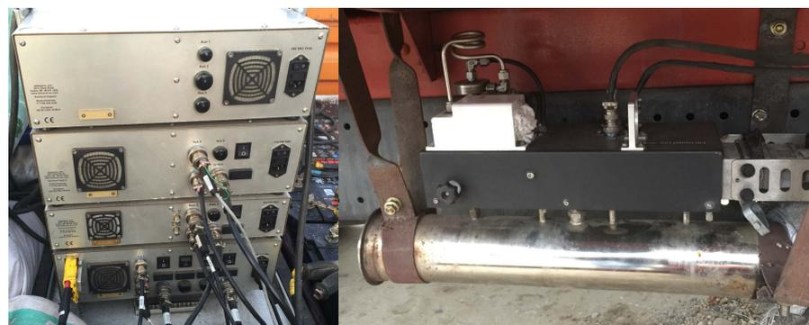
**Figure 2.** PEMS installed in dump trucks. The left is the gas analyzer units for measuring pollutants in the diluted exhaust; the right shows the sampling probes on the tailpipe with an exhaust mass flow meter.
