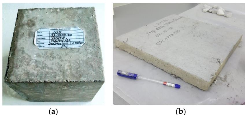
**Figure 6.** Specimens' geometry for thermal testing: (a) cube concrete specimen with a dimension of  $150 \times 150 \times 150$  mm for testing in accordance with ASTM D5334-14 and (b) plate concrete specimen with a dimension of  $40 \times 300 \times 300$  mm for testing in accordance with ASTM C518-15.
