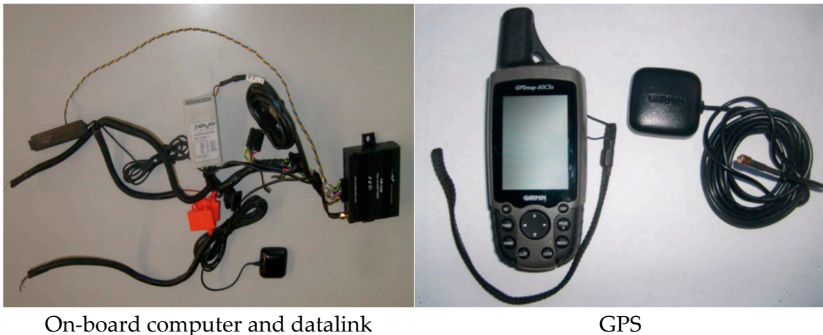
Figure 7. On-board computer and GPS used in the research.
