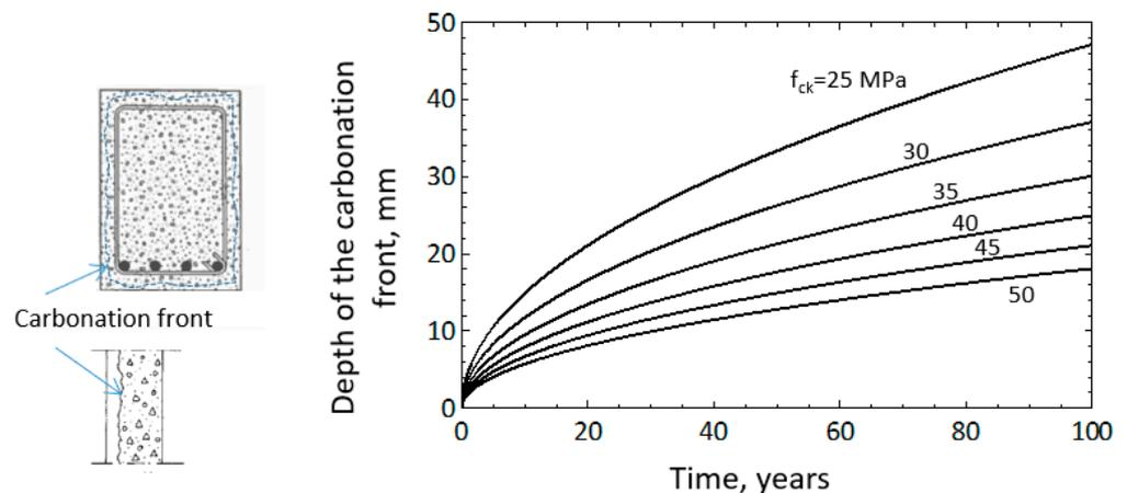
**Figure 2.** Depth of the carbonation front as a function of time.
