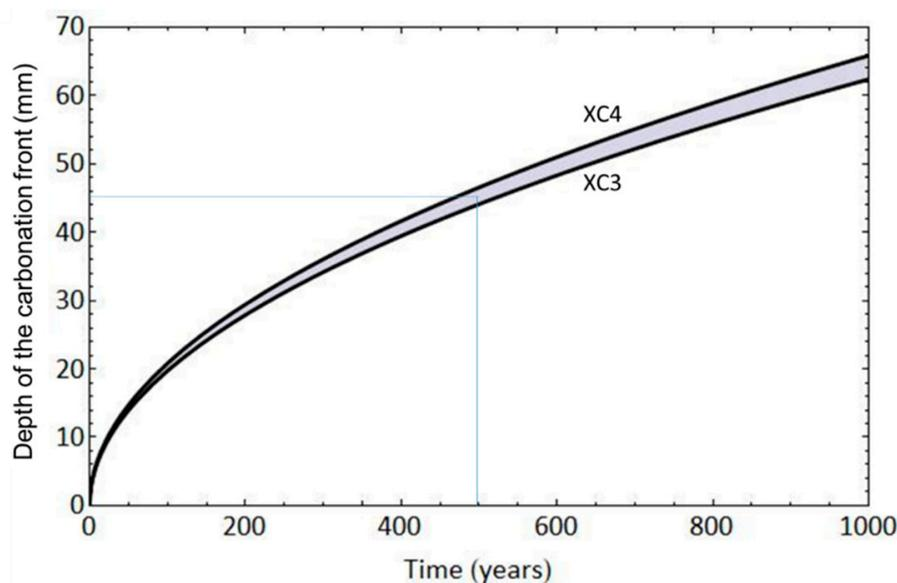
**Figure 7.** Expected service life of the Green Tunnel.
