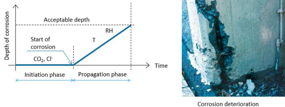
**Figure 1.** Conceptual scheme of a reinforcement corrosion process as a function of time, adapted from [7].
