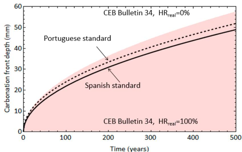
**Figure 4.** Comparison of the evolution of the carbonation front for Portland cement according to the Spanish Structural Code [35] and the Portuguese standard LNEC E-465 [28] for XC3 exposure class,  $c_{air} = 1.0$ , and  $f_{ck} = 50$  MPa. The range of values of the carbonation depth according to Annex C of CEB Bulletin 34 [36] for  $h_{Nd} = 182$  days,  $p_{sR} = 0$  for  $HR_{real}$  ranging between 0 and 100% is shown as a shaded area.
