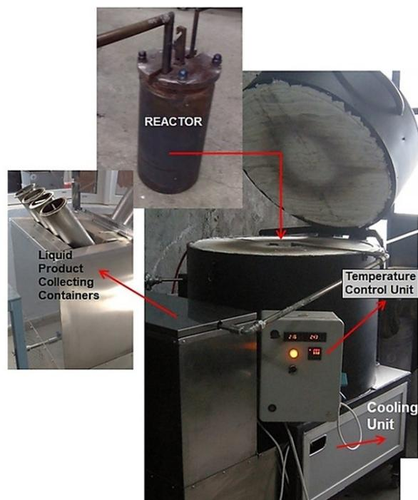
Figure 1. Pyrolysis system.
