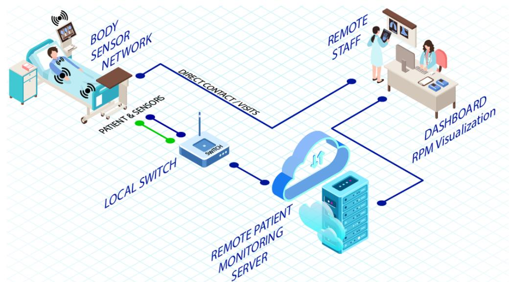
**Figure 1.** Architecture of a generic remote patient monitoring system [1].
