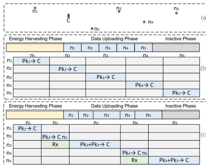
Figure 2. Illustration of the superframe, (a) Network, (b) Initialize phase, (c) Cooperation phase.
