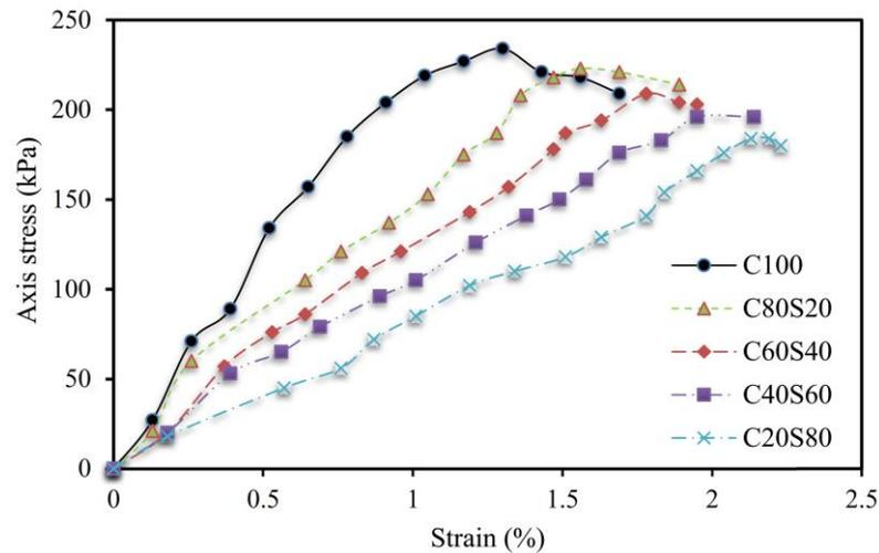
**Figure 3.** Unconfined compressive strength against axial strain.
