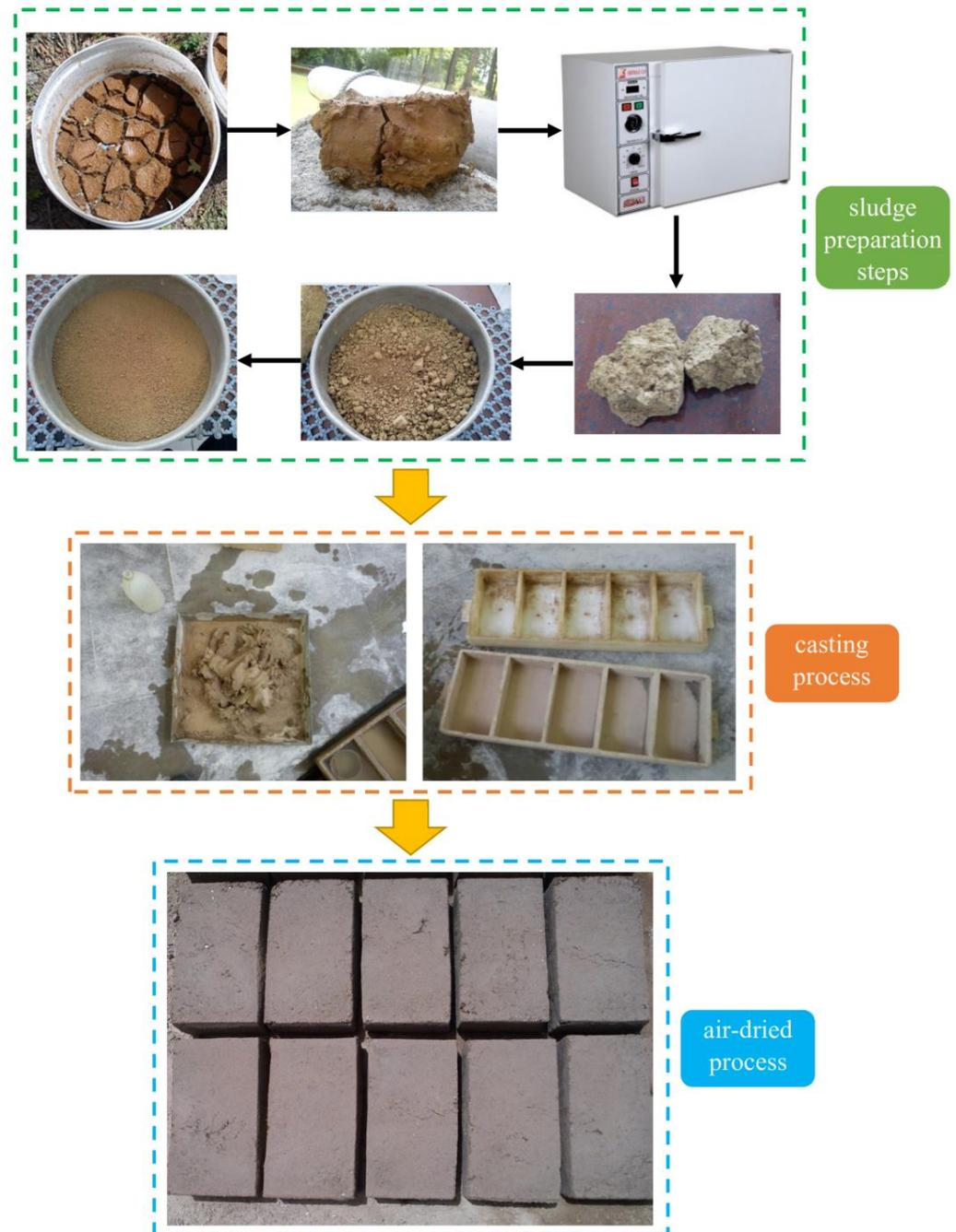
**Figure 1.** The brick preparation steps.
