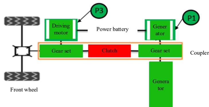
**Figure 5.** Series–parallel hybrid electric vehicle with a P1 + P3 structure.
