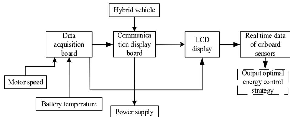
**Figure 4.** Energy consumption control structure of a hybrid electric vehicle.
