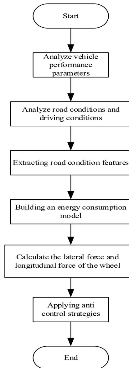
**Figure 1.** Energy consumption prediction algorithm flow for hybrid electric vehicles.
