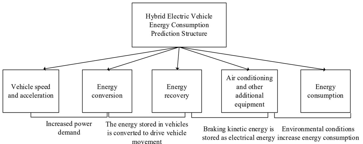
**Figure 2.** Energy consumption prediction structure of a hybrid electric vehicle.
