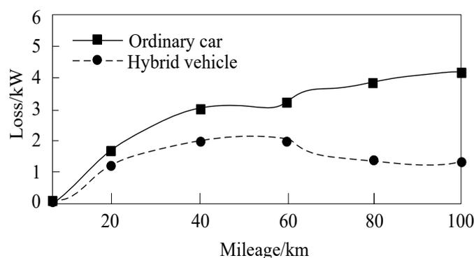
**Figure 6.** Test results of the different automobiles' driving energy consumption.
