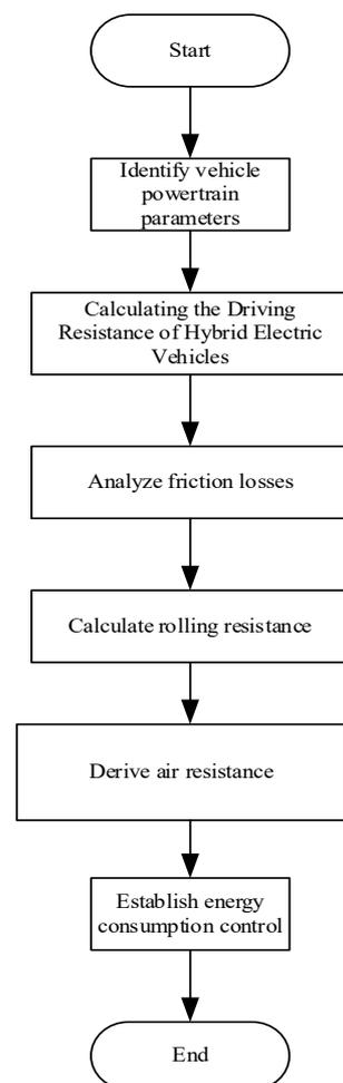
**Figure 3.** Energy consumption control algorithm flow for hybrid electric vehicles.
