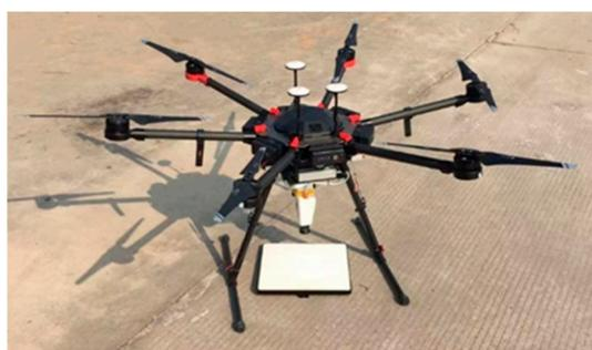
**Figure 2.** UAV-based hyperspectral observation platform and the white diffuse reflectance standard.
