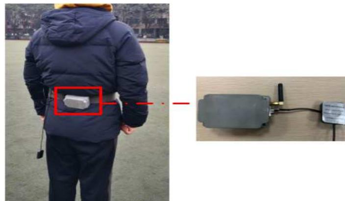
Figure 6. Integrated navigation system prototype display diagram and wearing diagram.
