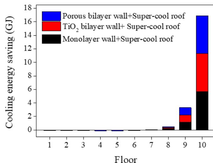
**Figure 10.** Super-cool-roof-induced cooling energy saving relative to the monolayer, TiO<sub>2</sub> bilayer, and porous P(VdF-HFP)-based bilayer walls without combining the super-cool roof.
