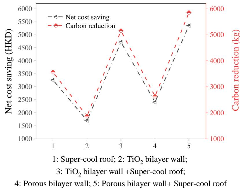
**Figure 13.** Annual net cost saving and carbon-emission reduction relative to the monolayer wall.
