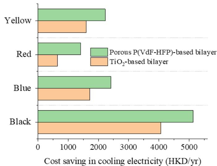
**Figure 8.** Net cost saving in cooling electricity induced by colored cooling walls relative to the monolayer.
