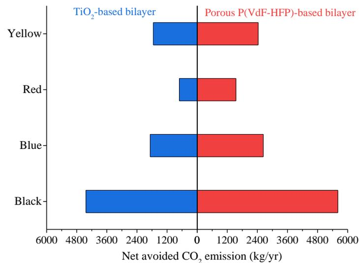
**Figure 9.** Net avoided CO<sub>2</sub> emission relative to the monolayer.
