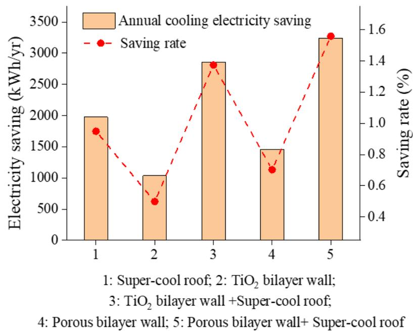
Figure 12. Yearly cooling electricity saving and saving rate relative to the monolayer wall.
