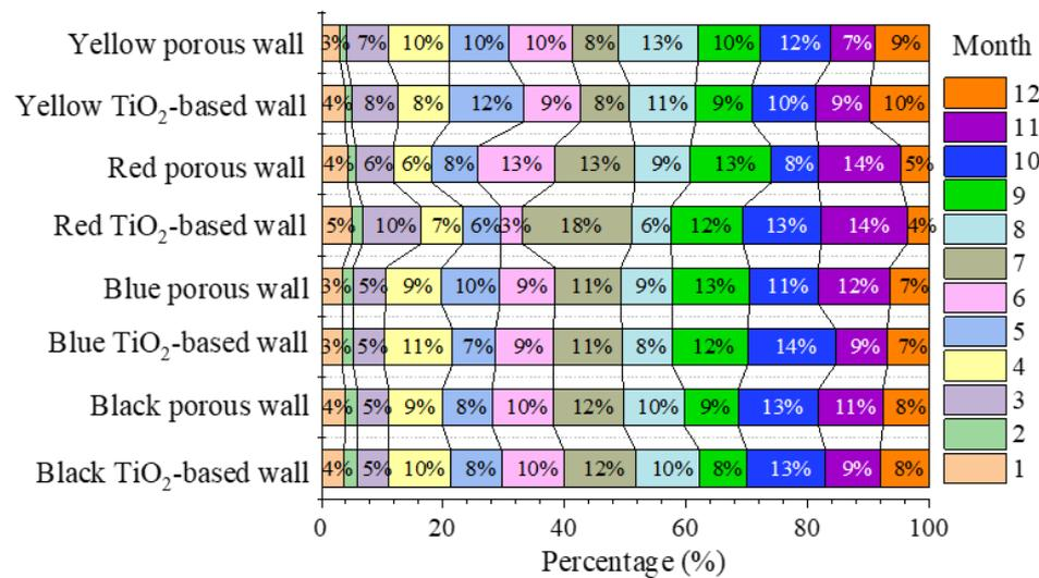
**Figure 7.** Percentage of monthly cooling energy saving distribution of differently colored cooling walls.
