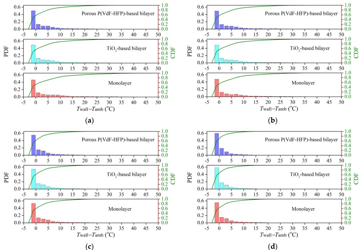
**Figure 3.** Statistical thermal analyses of differently colored walls relative to the ambient temperatures (a) Black wall. (b) Blue wall. (c) Red wall. (d) Yellow wall.
