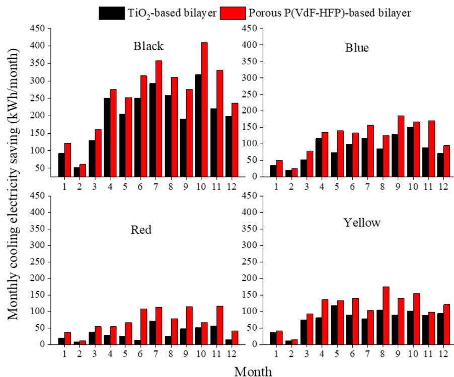
Figure 6. Monthly cooling energy saving distribution of differently colored cooling walls.
