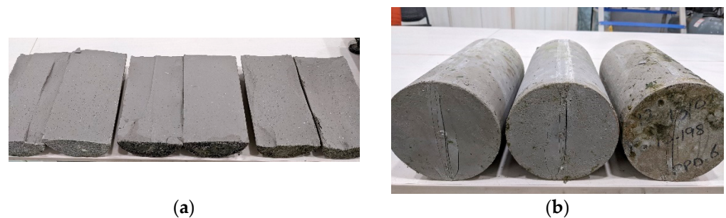
Figure 15. Sample pictures of specimen failure due to tensile stress for (a) PPF0 and (b) all TMs.
