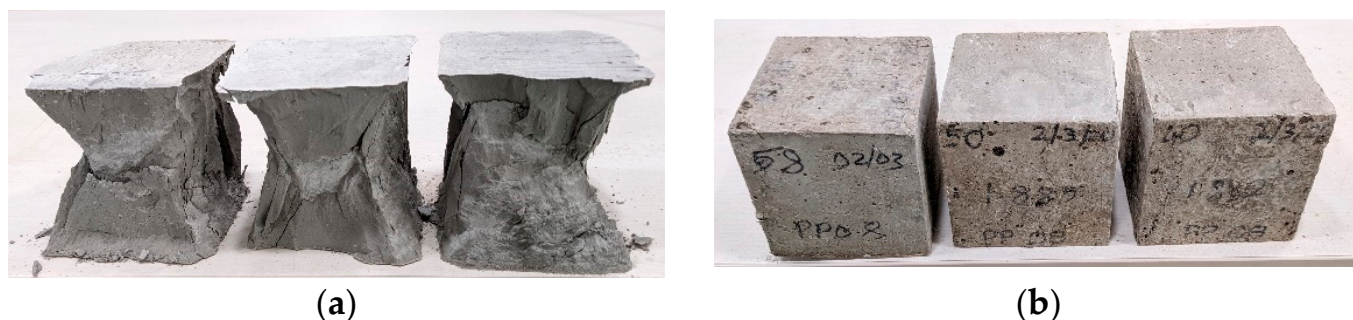
Figure 13. Typical specimen failure due to compressive stress for (a) PPF0 and (b) all TMs.
