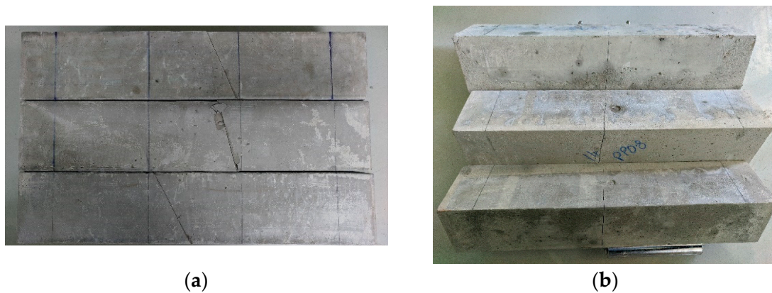
Figure 14. Sample pictures of specimen failure due to flexure stress for (a) control mix and (b) test mix.
