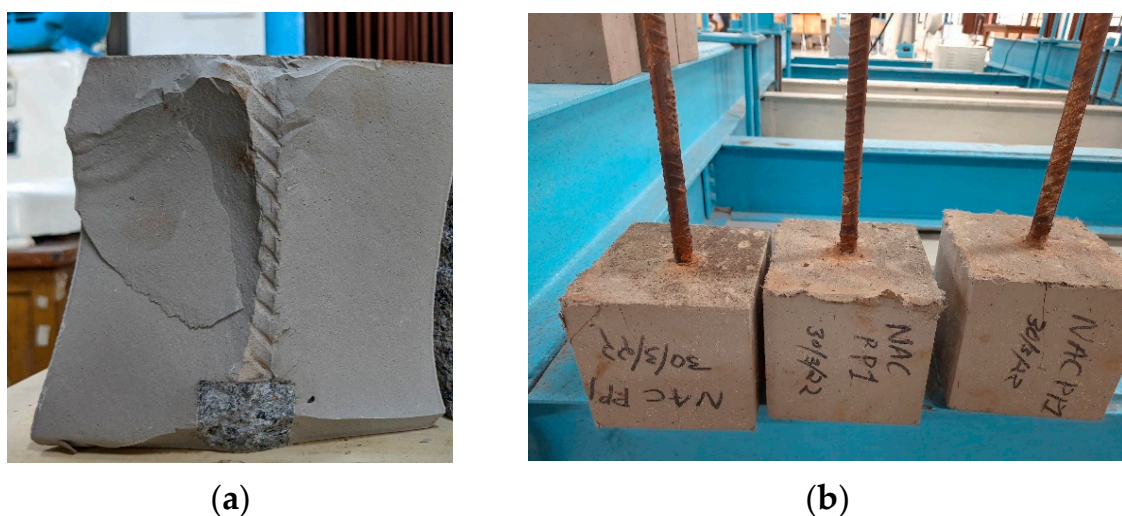
Figure 16. Sample pictures of specimen failure due to tensile stress for (a) PPF0 and (b) PPF1.0.
