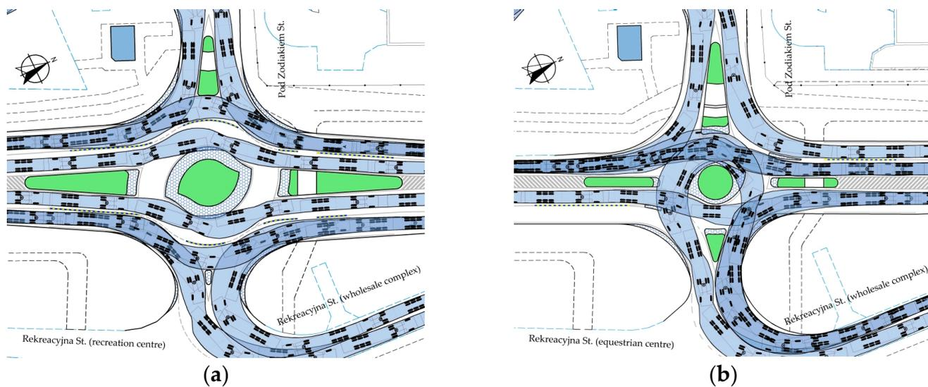
**Figure A6.** Examples of swept path analysis for “flattened” roundabouts with straight-through movements from the main approach legs plus right-turn movements: (a) with two exit lanes on the main approach legs—I type; (b) with one lane on the main approach legs—II type. Source: own work.
