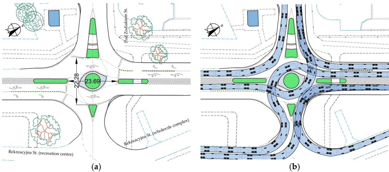
**Figure 20.** Example of “flattened” turbo-roundabout with a single traffic lane on the main road approach leg, recommended for areas of low urbanisation degree LUDA—single-family neighbourhoods or woonerf: (a) roundabout; (b) swept path DV2. Source: own work.
