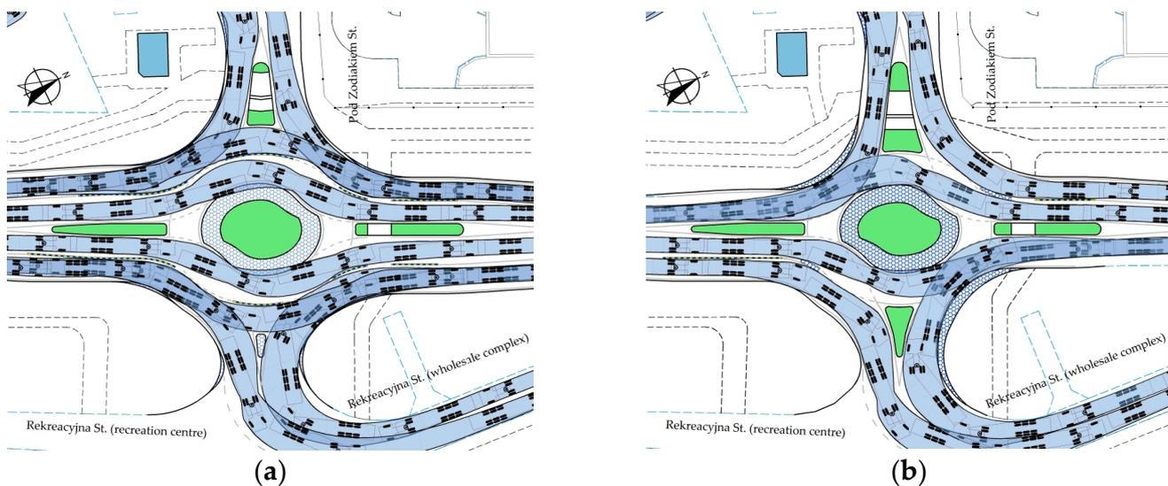
**Figure A7.** Examples of swept path analysis for elliptical turbo roundabouts with straight-through movements from the main approach legs plus right-turn movements: (a) with two exit lanes on the main approach legs—III type; (b) with one lane on the main approach legs—IV type. Source: own work.
