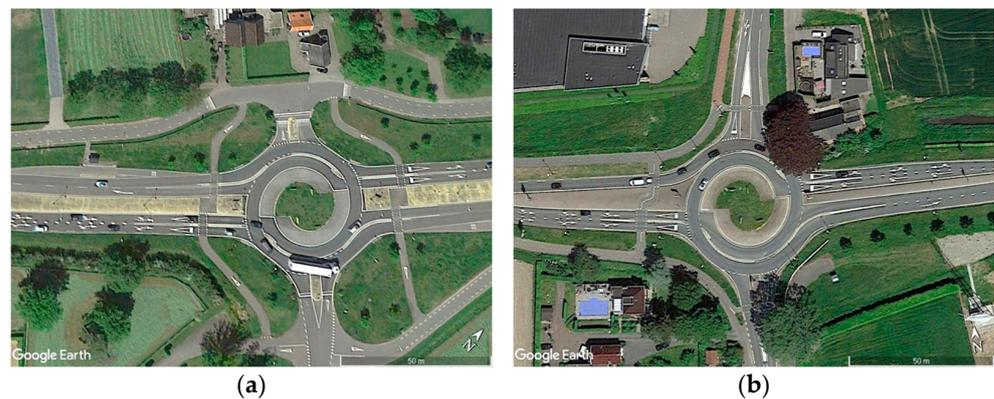
**Figure 1.** Examples of standard egg turbo-roundabouts located in constrained areas in the vicinity of buildings in The Netherlands: (a) Wierden ( $52^{\circ}20'39.79''$  N,  $6^{\circ}34'23.27''$  E); (b) Krimpen aan den IJssel ( $51^{\circ}48'36.17''$  N,  $4^{\circ}26'7.30''$  E). (Source: Google Earth [11]).
