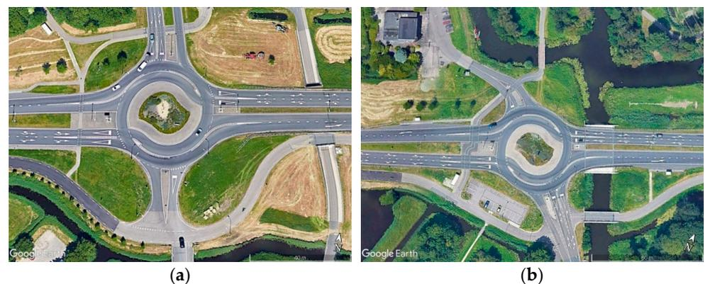
**Figure 2.** Examples of standard egg turbo-roundabouts located in constrained areas near lakes or canals in The Netherlands: (a) Wierden ( $51^{\circ}54'43.29''$  N,  $4^{\circ}38'34.10''$  E); (b) Krimpen aan den IJssel ( $51^{\circ}54'29.61''$  N,  $4^{\circ}37'23.73''$  E). (Source: Google Earth [11]).
