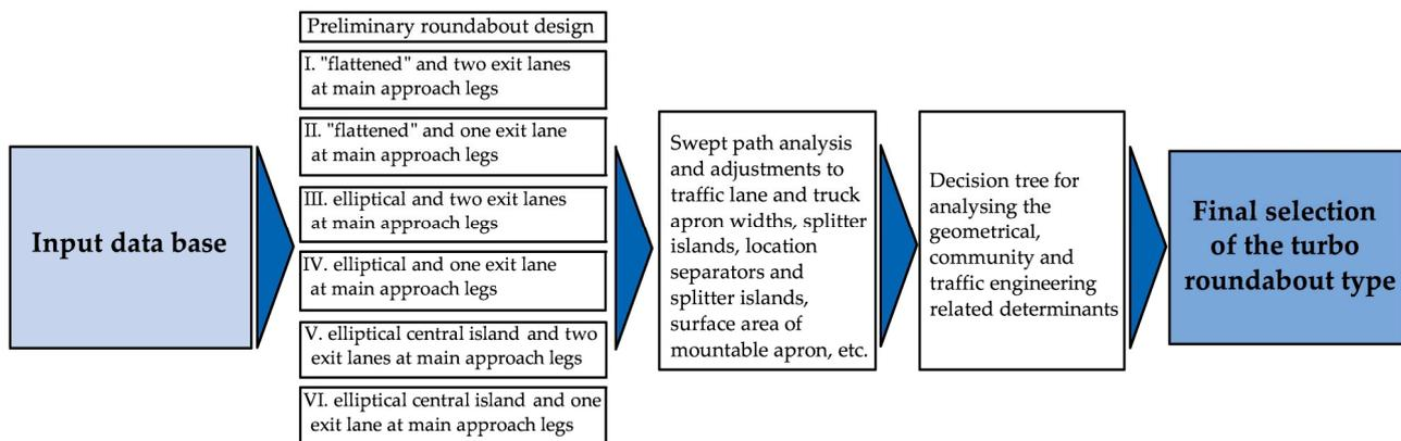
**Figure 9.** Nonstandard turbo-roundabout step-by-step selection diagram for constrained project sites.
