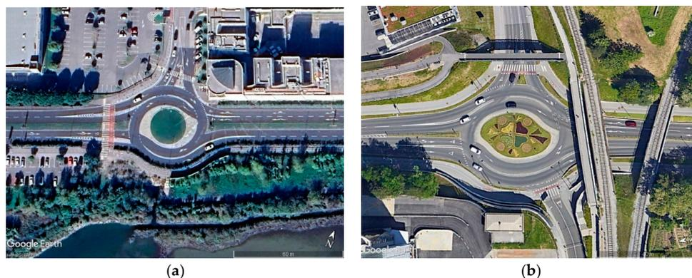
**Figure 3.** Examples of non-standard “flattened” turbo-roundabouts located in a constrained, built-up area in Slovenia: (a) Koper ( $45^{\circ}32'33.37''$  N,  $13^{\circ}44'21.78''$  E); (b) Maribor ( $46^{\circ}33'4.09''$  N,  $15^{\circ}38'59.64''$  E). (Source: Google Earth [11]).
