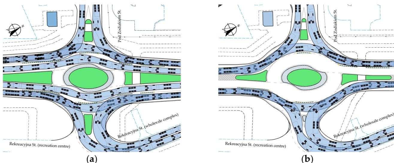
**Figure A8.** Examples of swept path analysis for elliptical turbo roundabouts featuring an elliptical central island with straight-through movements from the main approach legs plus right-turn movements: (a) with two exit lanes on the main approach legs—V type; (b) with one lane on the main approach legs—VI type. Source: own work.
