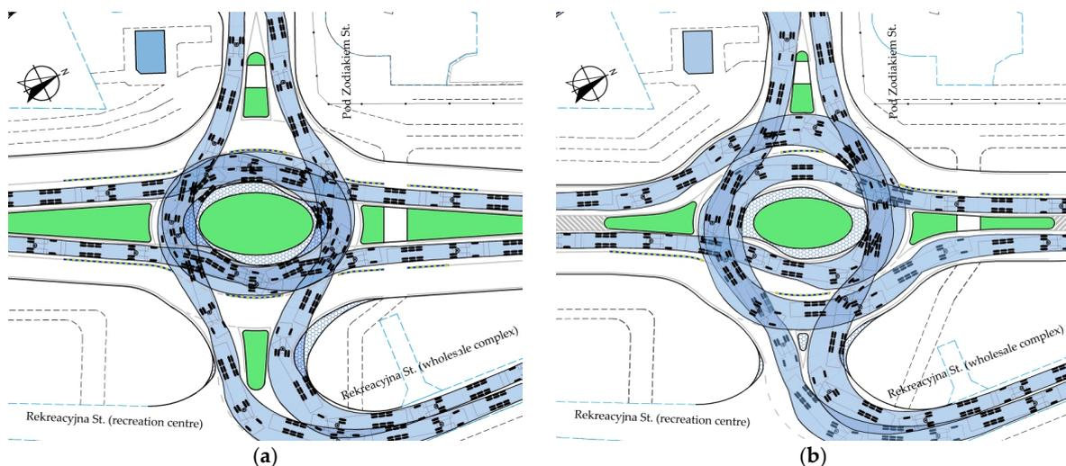
**Figure 18.** Examples of swept path analyses for elliptical roundabouts featuring an elliptical central island: (a) with two exit lanes on the main approach legs—V type; (b) with one lane on the main approach legs—VI type. Source: own work.
