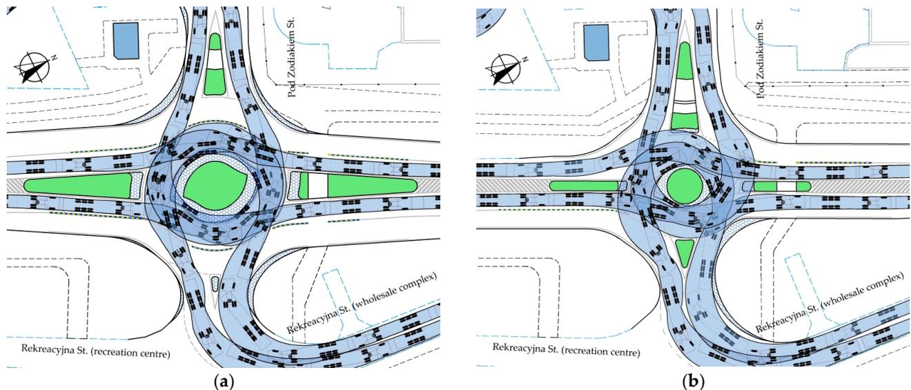
**Figure 12.** Examples of swept path analyses for “flattened” roundabouts left-turn movements: (a) with two exit lanes on the main approach legs—I type; (b) with one lane on the main approach legs—II type. Source: own work.
