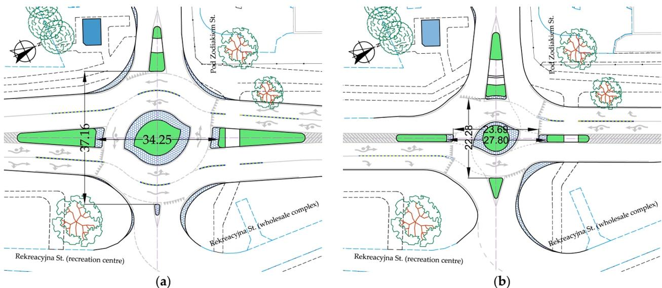
**Figure 11.** Examples of “flattened” roundabouts: (a) with two exit lanes on the main approach legs—I type; (b) with one lane on the main approach legs—II type. Source: own work.
