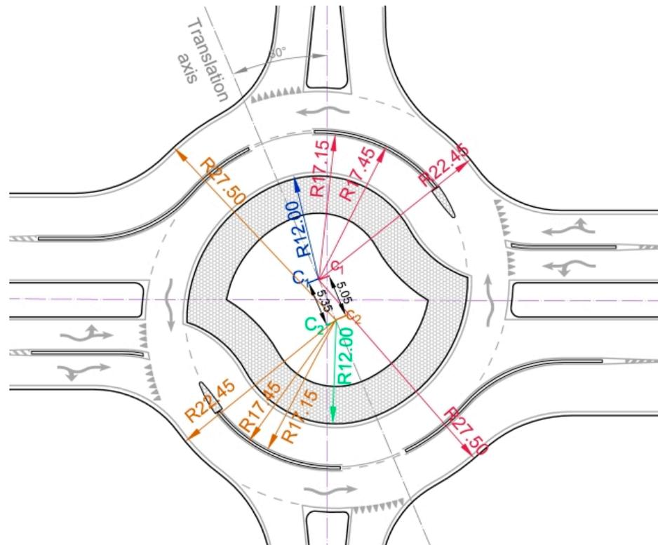
Figure A5. Turbo block of a standard small egg turbo roundabout.
