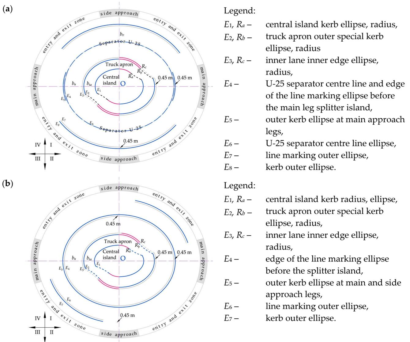
**Figure 13.** One exit lane at main approach legs. Turbo block for laying out elliptical turbo-roundabouts: (a) with two exit lanes on the main approach legs—III type; (b) with one lane on the main approach legs—IV type. Source: own work.
