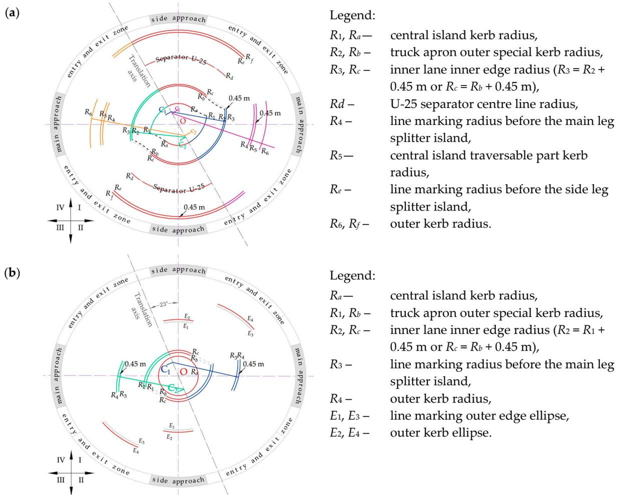
**Figure 10.** Turbo block to layout “flattened” roundabouts: (a) with two exit lanes on the main approach legs—I type; (b) with one lane on the main approach legs—II type. Source: own work. The
