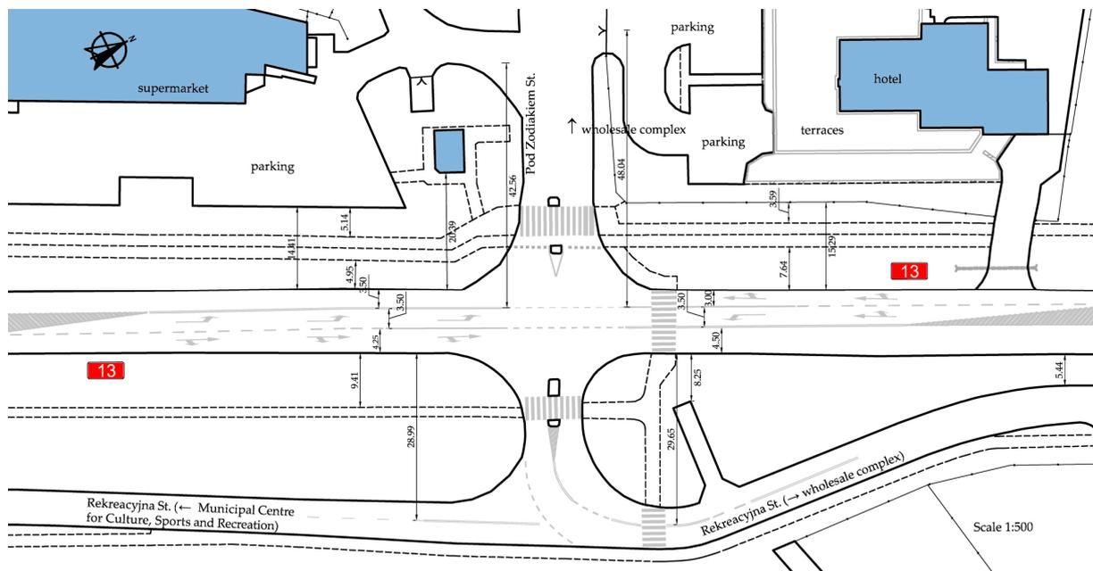
Figure A1. Illustrative junction layout plan showing site constraints—case study; distance to the junction to the south—184 m; distance to the junction to the north—234 m (all distances are in metres).
