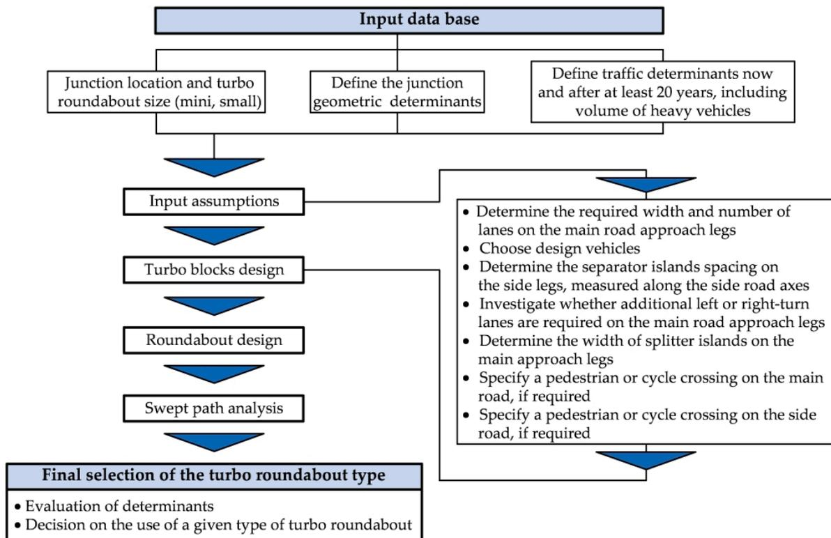
Figure 4. The turbo roundabout selection method for constrained areas is presented in the diagram.
