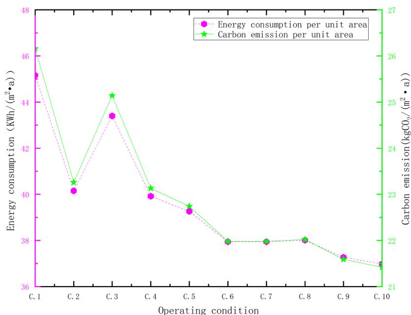
**Figure 8.** Unit area energy consumption and carbon emission results.
