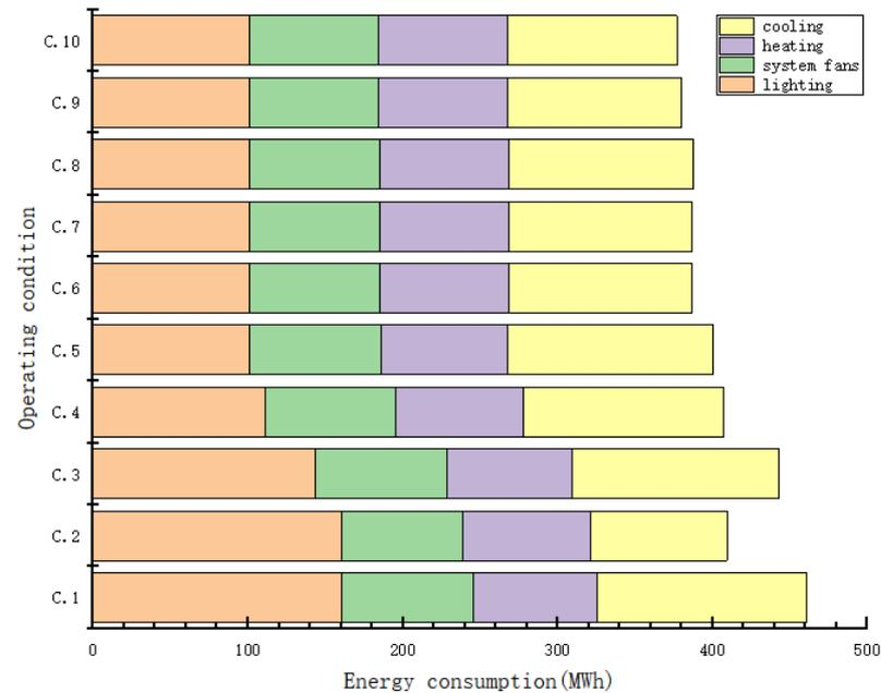
**Figure 7.** Annual sub-energy consumption simulation results.
