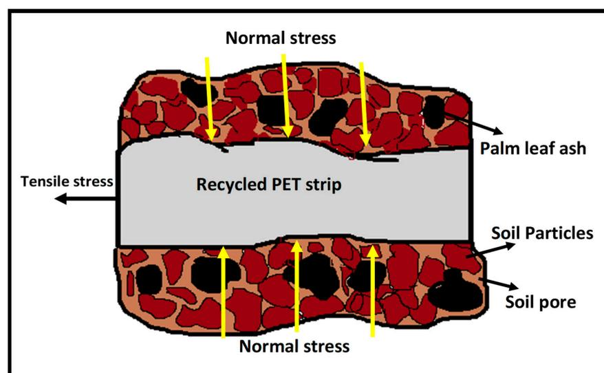
Figure 8. The interaction mechanism between PLA, PET strips, and soil particles.
