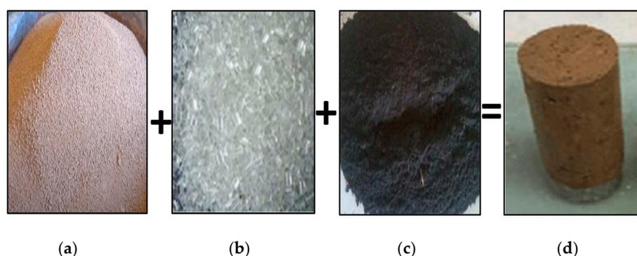
**Figure 3.** Mixing of (a) clayey sand, (b) recycled PET, and (c) palm leaf ash to make (d) the soil-reinforced sample.
