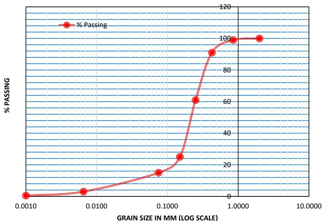
**Figure 1.** Particle size distribution curve for soil sample.
