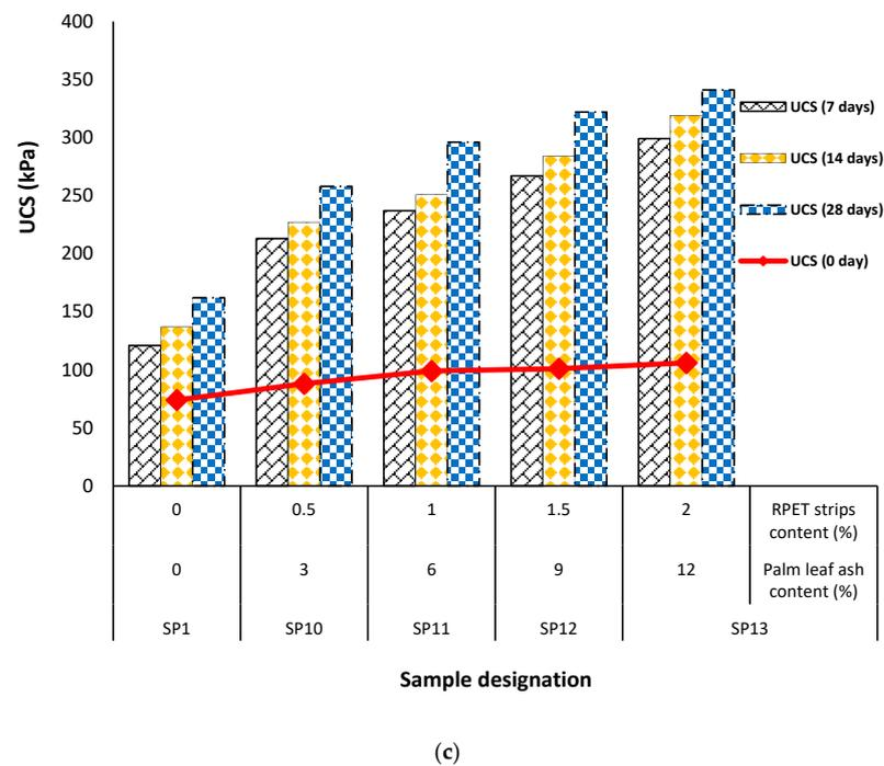
**Figure 5.** Influence of recycled PET strips with PLA on UCS of soil: (a) 10 mm recycled PET strip length, (b) 20 mm recycled PET strip length, (c) 30 mm recycled PET strip length.
