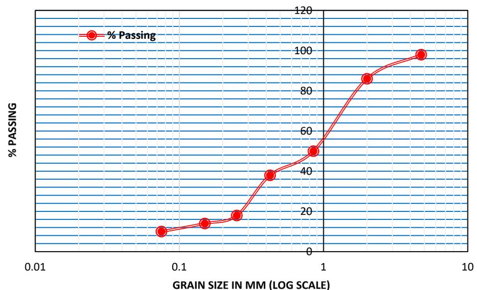
**Figure 2.** Particle size distribution curve for PLA.
