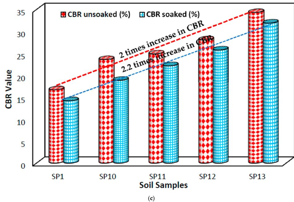
**Figure 7.** Influence of recycled PET strips with PLA on CBR value of soil samples: (a) 10 mm PET strip length, (b) 20 mm PET strip length, (c) 30 mm PET strip length.
