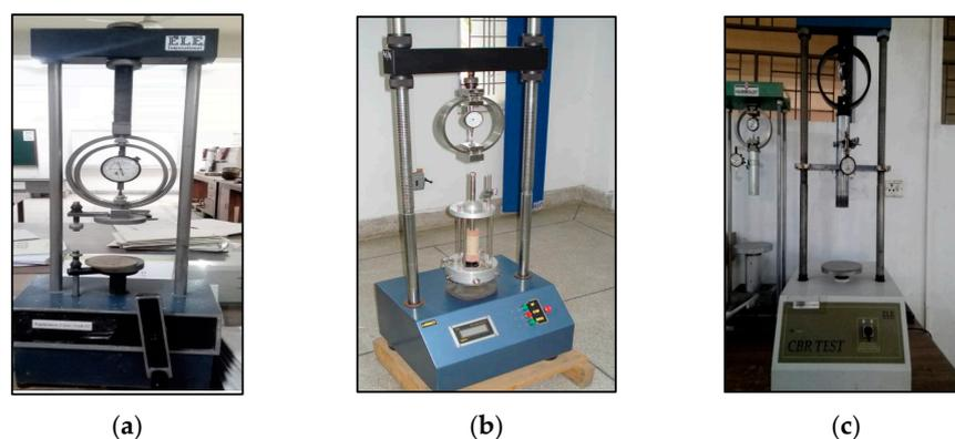
**Figure 4.** Test apparatus for (a) UCS, (b) triaxial, and (c) CBR.
