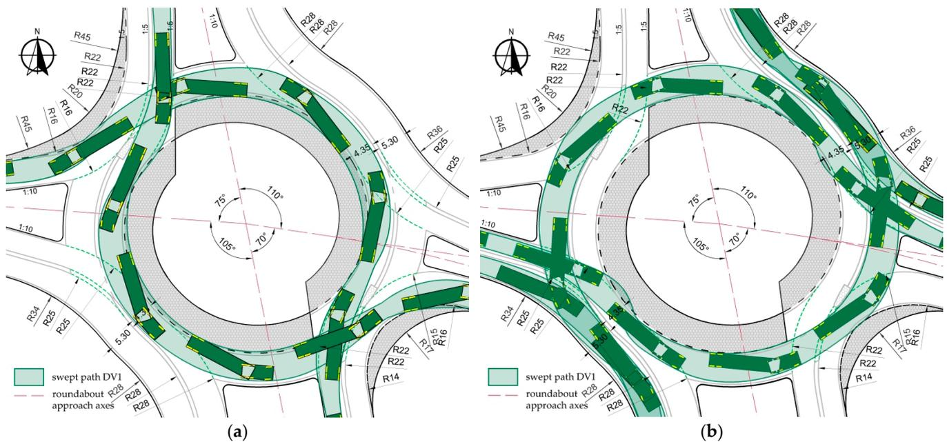
**Figure 14.** Swept paths of DV1: (a) for left-turning movements from the main approaches; (b) for right- and left-turning movements from the side approaches (units in m). Source: own work.
