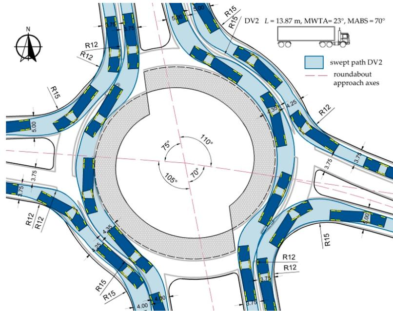
Figure A1. Selected swept paths of DV2—right-turning movement and straight-ahead movement—north and south approach (units in m). Source: own work.
