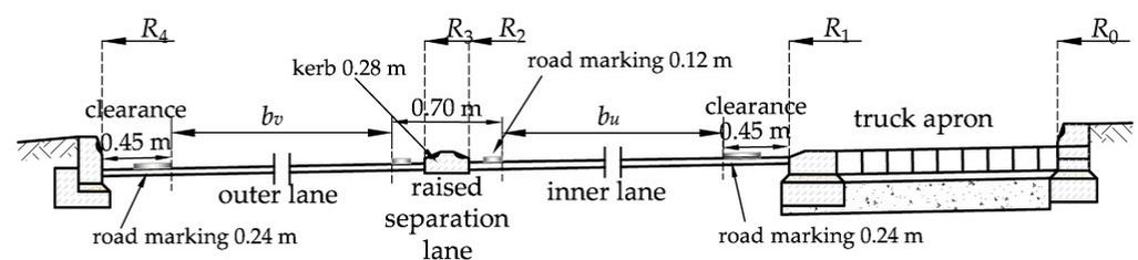
**Figure 2.** Lane widths and distances between edge lines in a turbo-roundabout. Source: own work.
