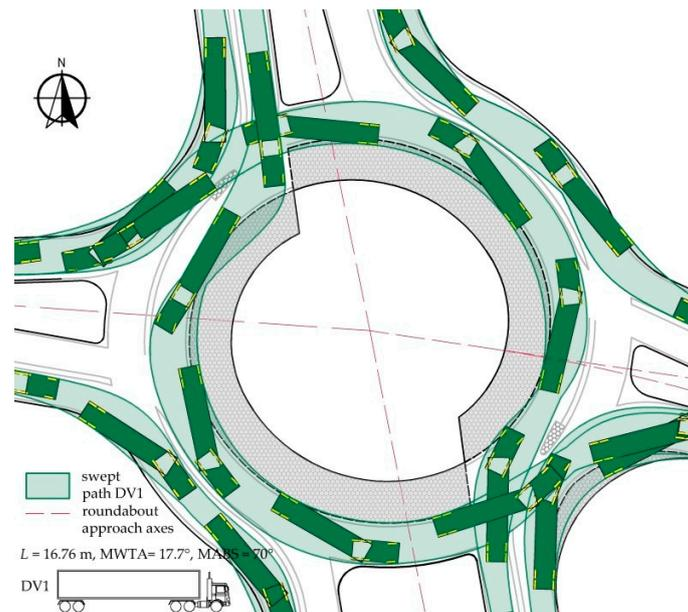
**Figure 11.** Selected swept paths of DV1 following a change in the roundabout geometry that involved primarily widening the circulatory lanes. Source: own work.
