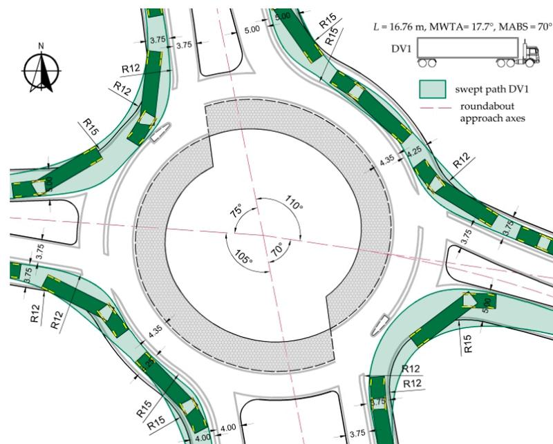
**Figure A4.** Selected swept paths of DV1—right-turning movement and necessity mountable aprons (units in m). Source: own work.
