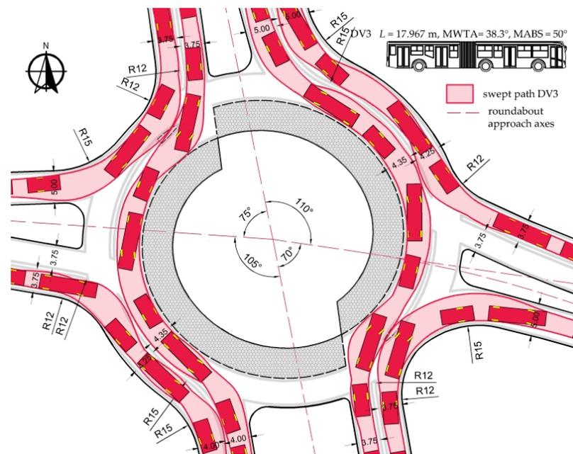
**Figure A3.** Selected swept paths of DV3—right-turning movement and straight-ahead movement—north and south approach (units in m). Source: own work.
