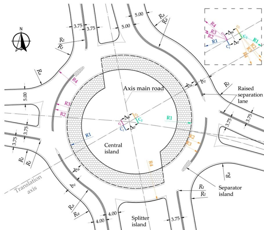
**Figure 3.** Turbo block of a standard turbo-roundabout *Basic* adjusted to the entries when the main traffic flow is north-south (units in m). Source: own work.
