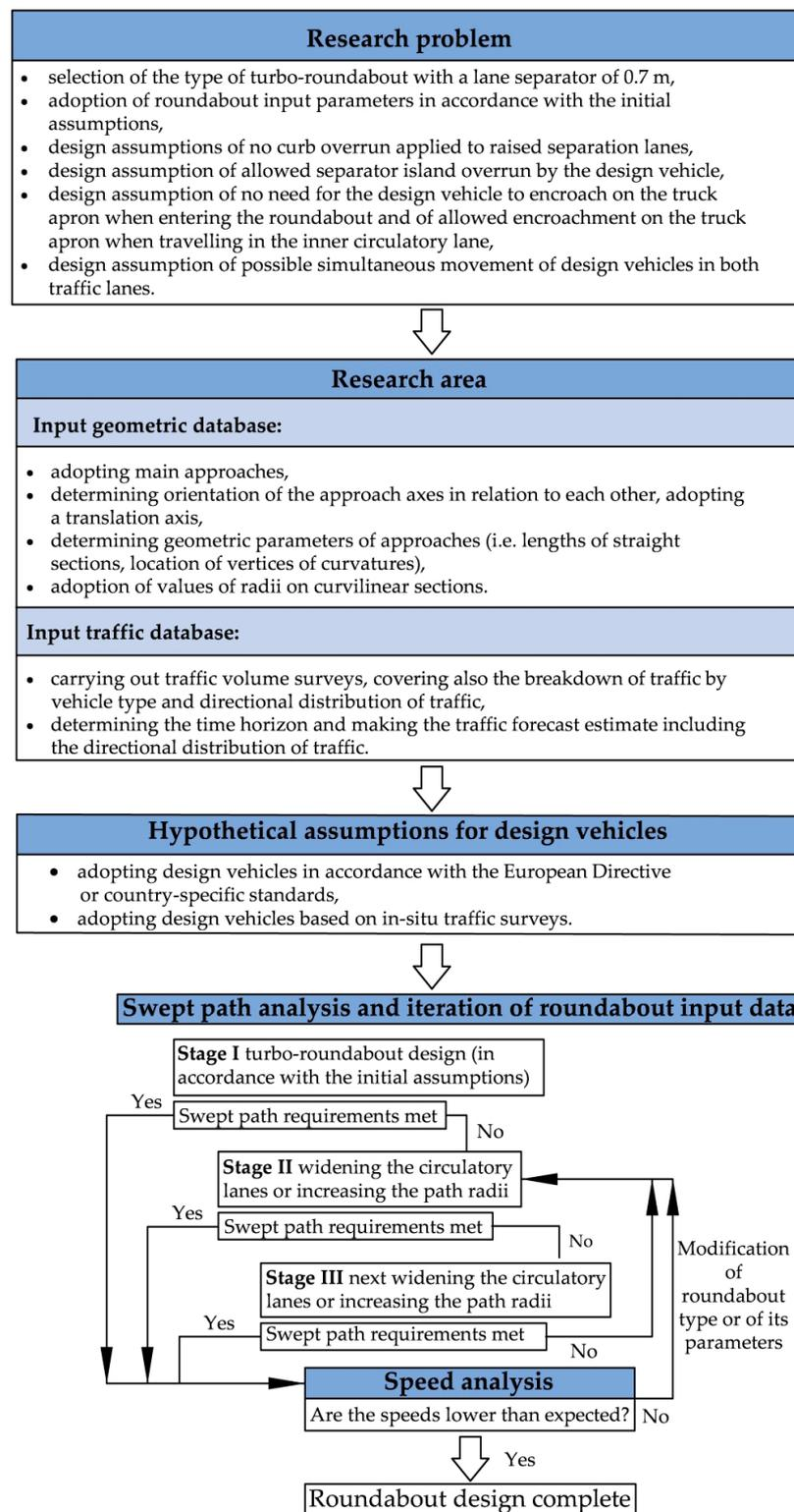
**Figure 6.** Step-by-step analysis method. Source: own work.
