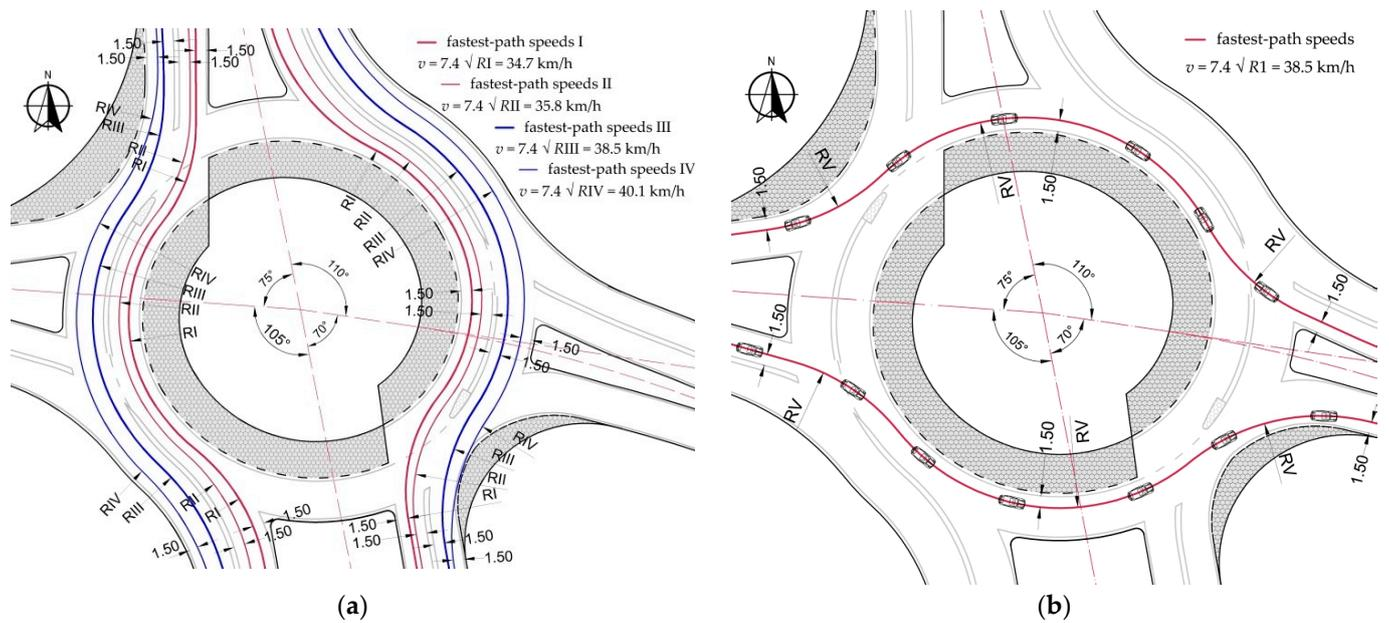
**Figure 15.** Fastest vehicle paths through the roundabout: (a) from the main approaches; (b) from the side approaches (units in m). Source: own work.
