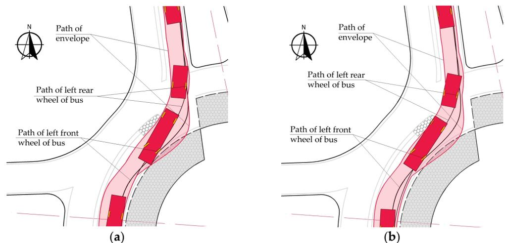
**Figure 10.** DV3 swept paths at the entry to the roundabout from the north approach leg: (a) left-turning movement; (b) straight-ahead movement. Source: own work.
