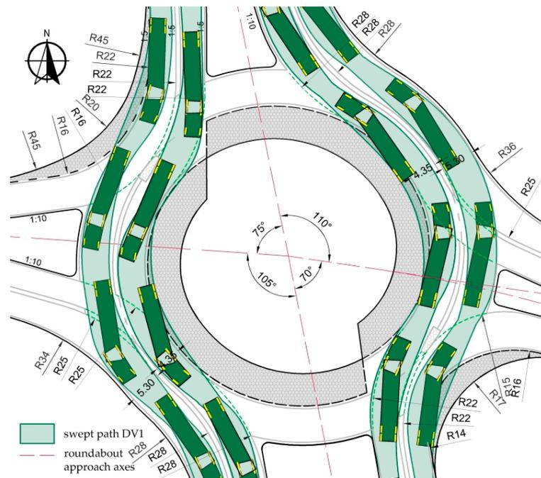
**Figure 13.** DV1 swept paths for the straight-ahead movements from the main approaches (units in m). Source: own work.
