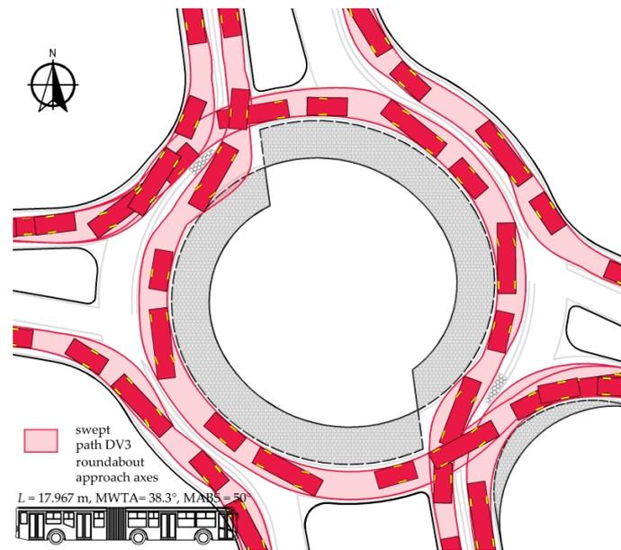
**Figure 9.** Selected DV3 swept paths following a change in the roundabout geometry that involved primarily widening the circulatory lanes. Source: own work.
