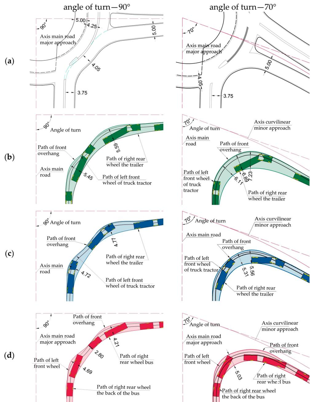
**Figure 5.** Minimum turning paths for the design vehicle during right turn at 70° and 90° angles: (a) fragment of the geometry of selected approaches; (b) swept path of design vehicle DV1; (c) swept path of design vehicle DV2; (d) swept path of design vehicle DV3 (units in m). Source: own work.
