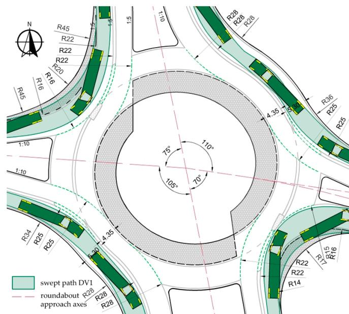
**Figure 12.** DV1 swept paths for right-turning movements (units in m). Source: own work.
