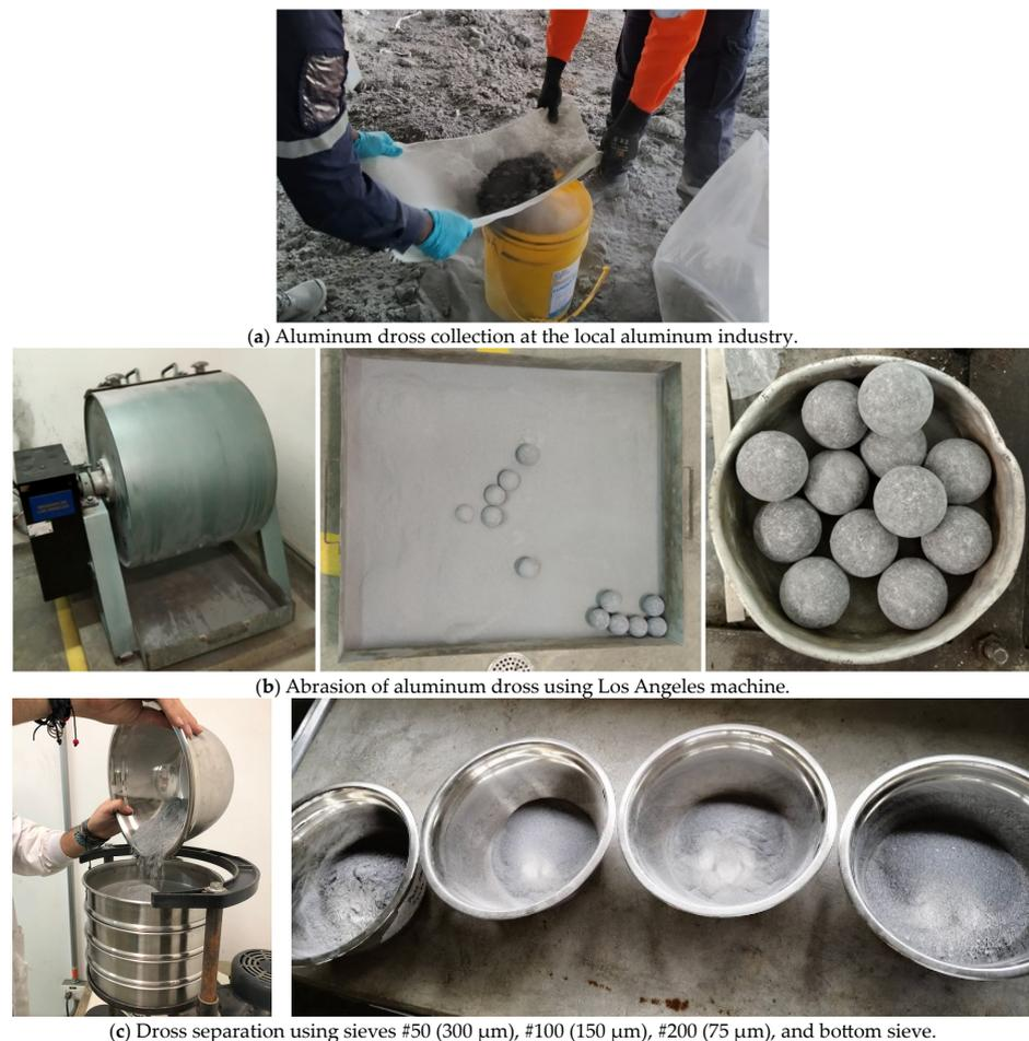
**Figure 3.** Aluminum dross collection and inactivation processes.
