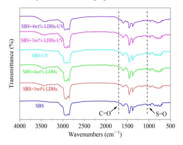
Figure 14. The FTIR spectra of MABs before and after UV aging.
