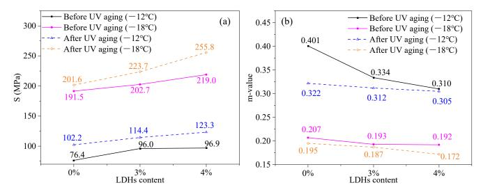
Figure 11. Low-temperature rheological properties of LDH MABs ((a) S, (b) m-value).
