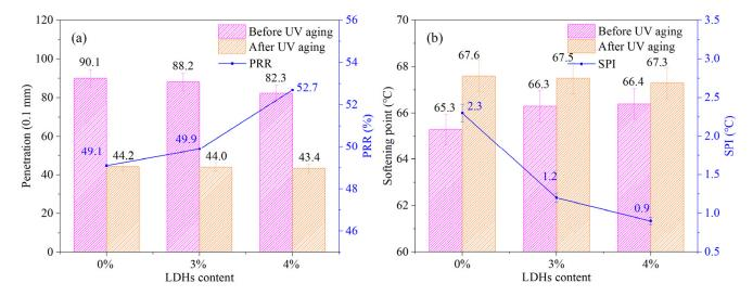
Figure 9. Effect of UV aging on (a) PRR (%) and (b) SPI (°C) of LDH MABs.
