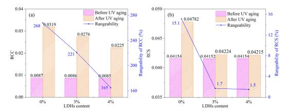
Figure 15. The RCC and RCS of MABs before and after UV aging ((a) RCC, (b) RCS).
