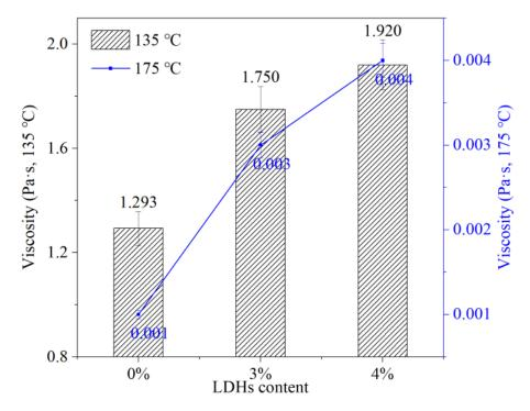
**Figure 8.** The viscosity of LDH MABs at 135 °C and 175 °C.
