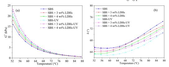
**Figure 13.** High-temperature rheological properties of LDH MABs with different LDH contents ((a) complex modulus, (b) phase angle).
