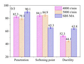
**Figure 6.** Effect of preparation parameters ((**a**) temperature, (**b**) time, (**c**) shearing rate) on 25 °C penetration, softening point, and 15 °C ductility of LDH MABs.
