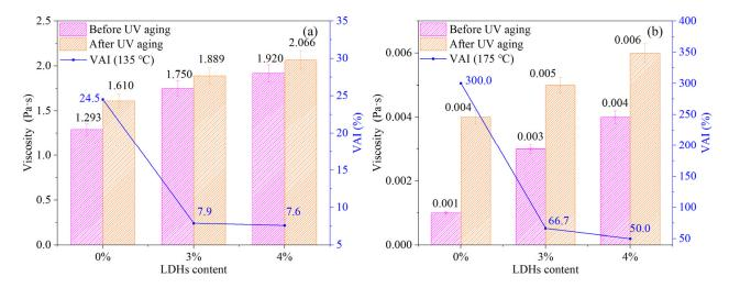
Figure 10. Effect of UV aging on the VAI (%) of LDH MABs ((a) 135 °C, (b) 175 °C).
