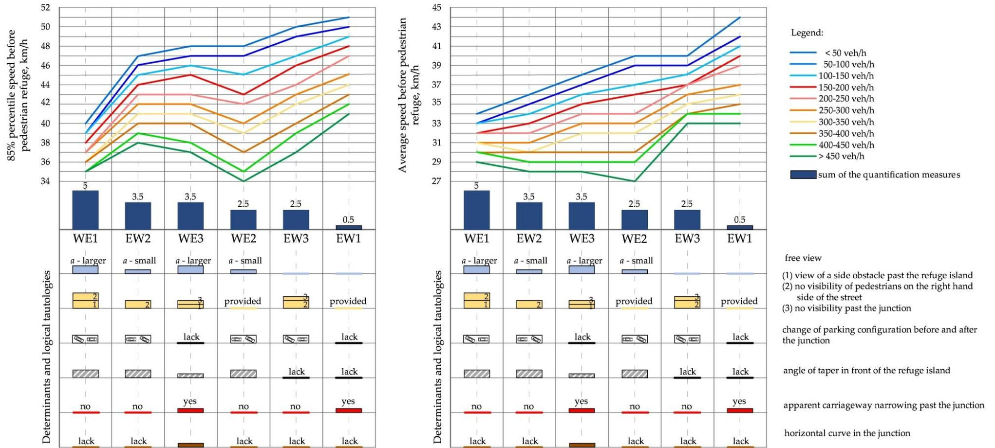
**Figure 13.** Pareto chart showing the variation of speed distribution parameters ( $v_{85}$  and  $v_{av}$ ) and the determinants adopted for the analysed sections: the sections are listed in the growing order of  $v_{85}$  just before the refuge island; and the test sections are listed in the order  $v_{av}$  just before the refuge island. Source: own work.
