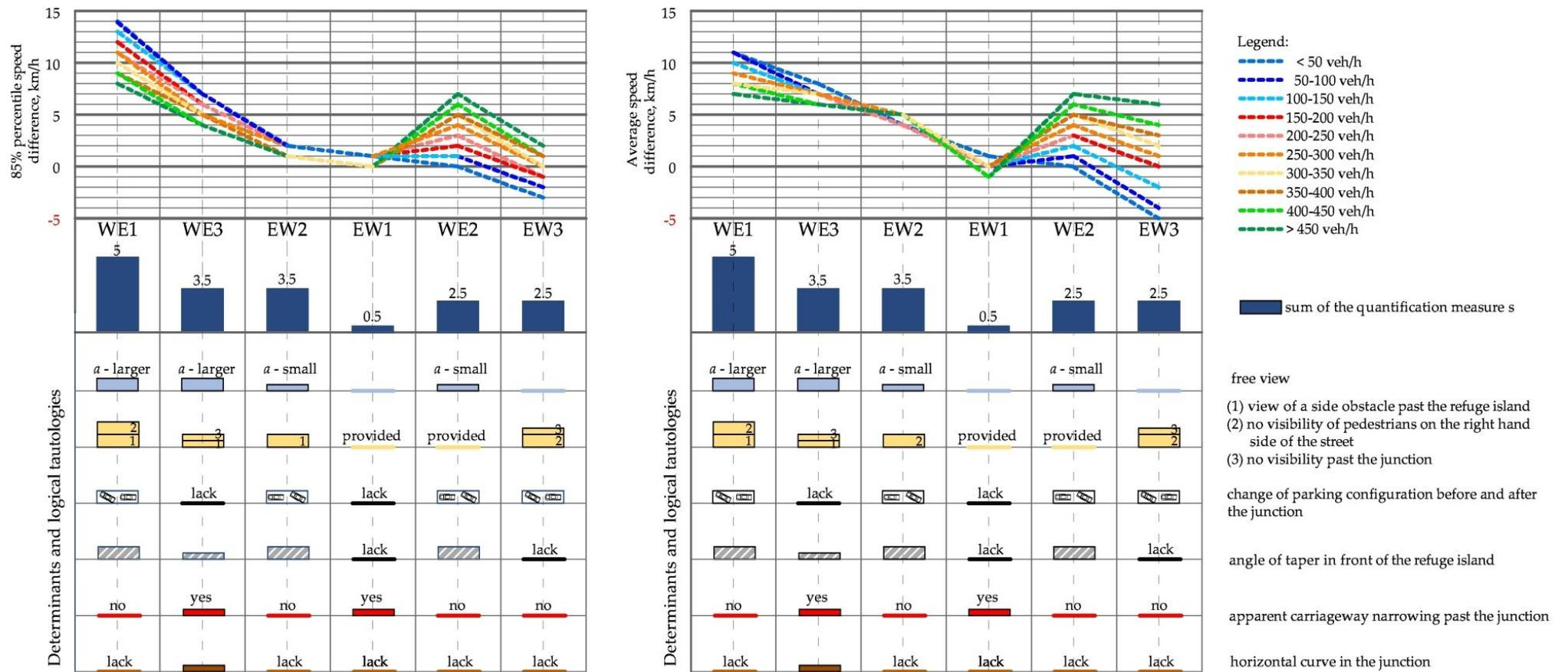
**Figure 14.** Pareto Chart 2—showing the values of  $\Delta v_{85}$  and  $\Delta v_{av}$  and the determinants adopted on the respective sections: sections listed in the order of  $\Delta v_{85}$  values calculated as  $\Delta v_{85} = v_{85}(\text{entry}) - v_{85}(\text{before the refuge island})$ ; and sections listed in the order of  $\Delta v_{av}$  values calculated as  $\Delta v_{av} = v_{av}(\text{entry}) - v_{av}(\text{before the refuge island})$ . Source: own work.
