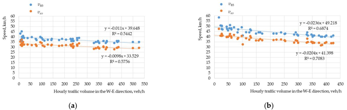
**Figure 9.** Regression analysis examples for different survey station locations: (a) at a refuge island; (b) on the refuge island approach section. Source: own work.
