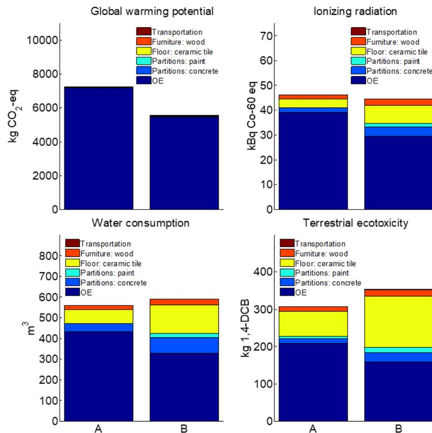
**Figure 2.** Energy<sub>Low</sub>–Materials<sub>High</sub> (A) and Energy<sub>High</sub>–Materials<sub>Low</sub> (B) LEED-CI v4 gold certification strategies with natural gas used for operational energy (OE) production.
