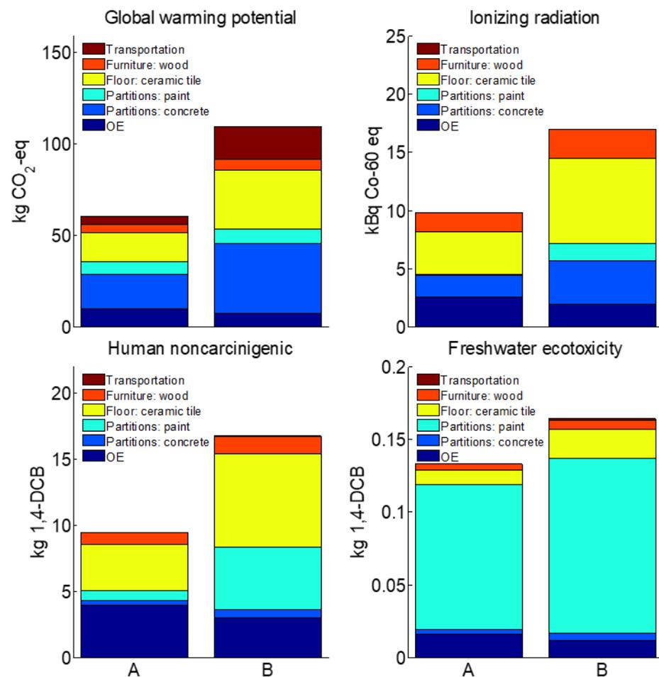
**Figure 3.** Energy<sub>Low</sub>-Materials<sub>High</sub> (A) and Energy<sub>High</sub>-Materials<sub>Low</sub> (B) strategies with photovoltaic (PV) energy used for operational energy (OE).
