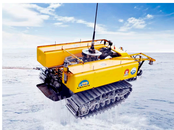
Figure 7. 514 m sea trial collection vehicle.
