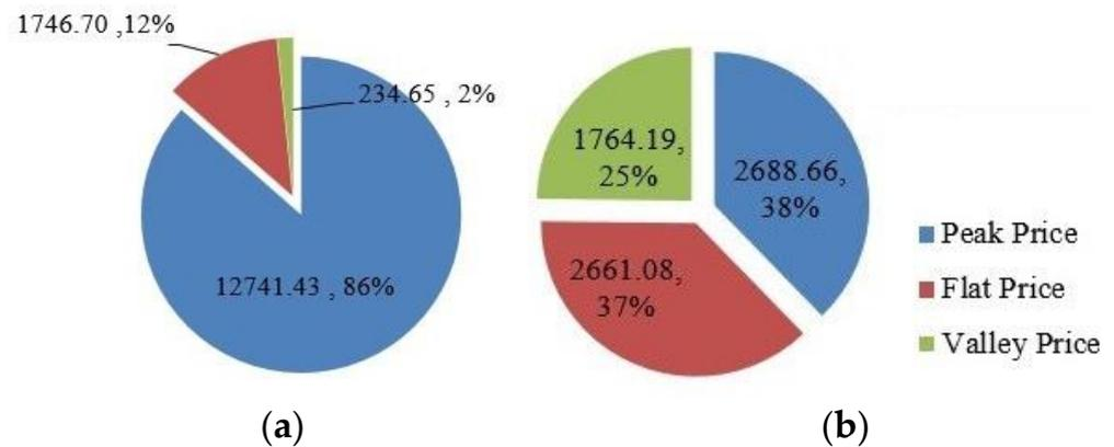
Figure 9. Distribution diagram of electricity charge before and after adding the energy storage device. (a) Electricity price without energy storage device; (b) electricity price with energy storage device.
