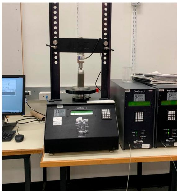
**Figure 5.** The setup of the UCS test.
