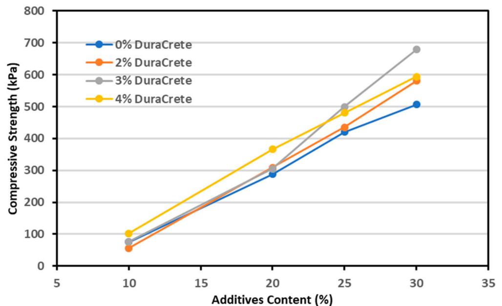
Figure 14. The effect of additives content on compressive strength.
