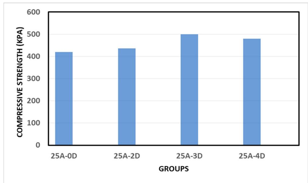
Figure 9. The compressive strength results of the specimens of 25% additives.
