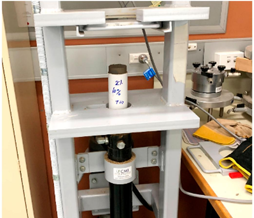
**Figure 11.** Extrusion of sample using hydraulic jack.
