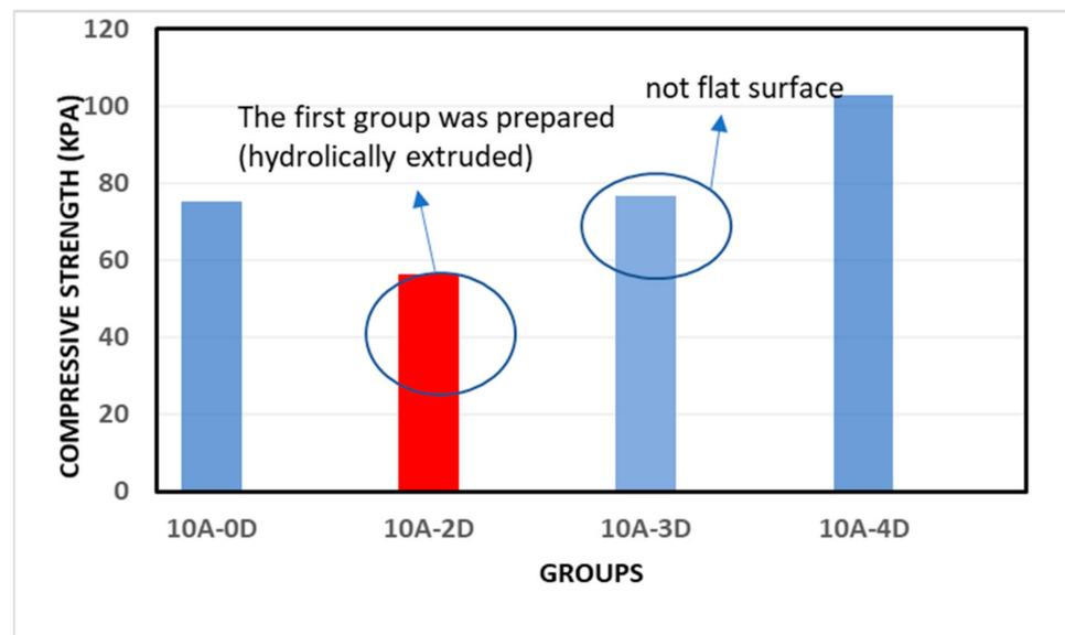
Figure 7. The compressive strength results of the specimens of 10% additives.
