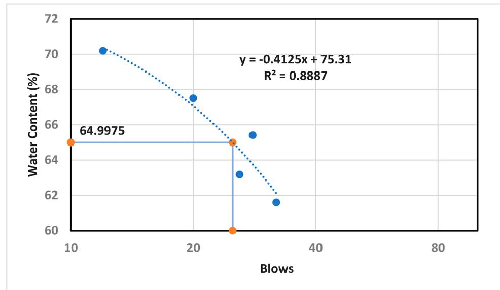
**Figure 6.** Linear fitting of the experimental data for liquid limit calculation (semi-log diagram).
