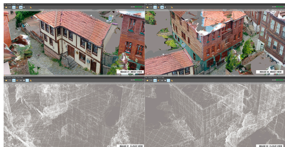
Figure 7. Point cloud visualization of Kapanca Street using Acute3D Viewer.
