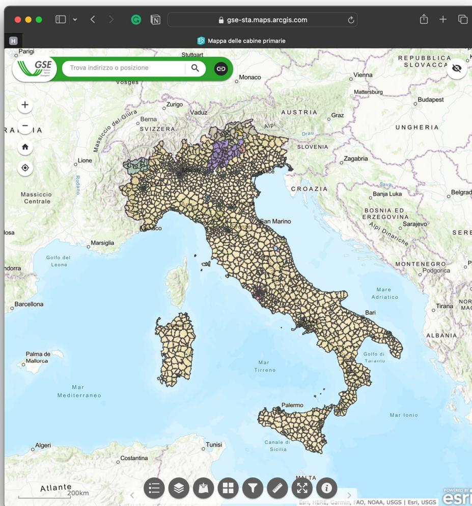
**Figure 3.** WebGIS provided by GSE for principal substation boundary identification. Given the plurality of energy distributors across the country, the ‘Aree Convenzionali’ layer shows with different colours the areas served by a different energy distributor.
