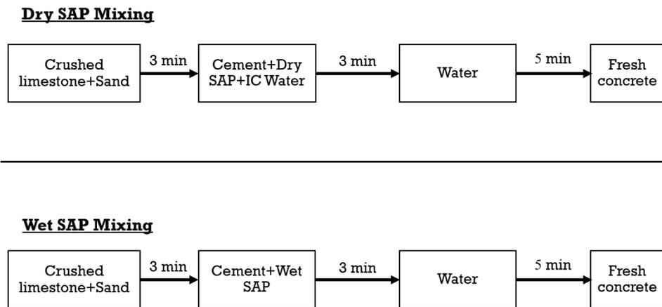
Figure 7. Mixing steps for concrete with SAP.
