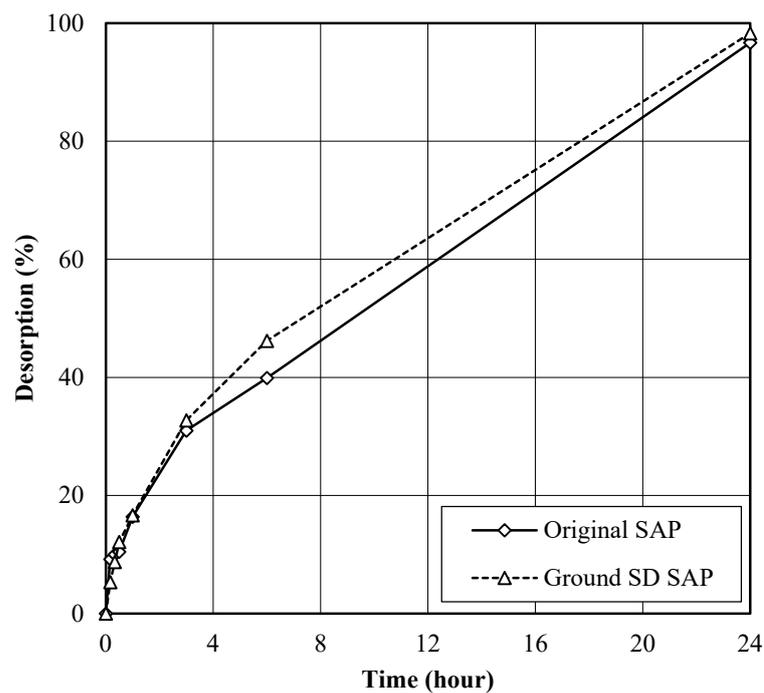
Figure 5. Desorption capacity of SAP.
