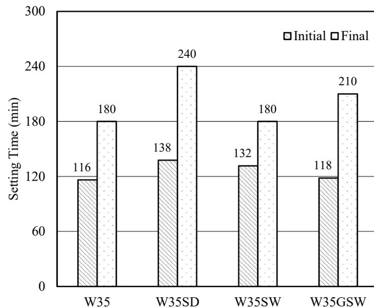
Figure 9. Setting time for mortar.
