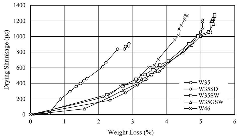
**Figure 14.** Relationship between the drying shrinkage and weight loss of mortar.
