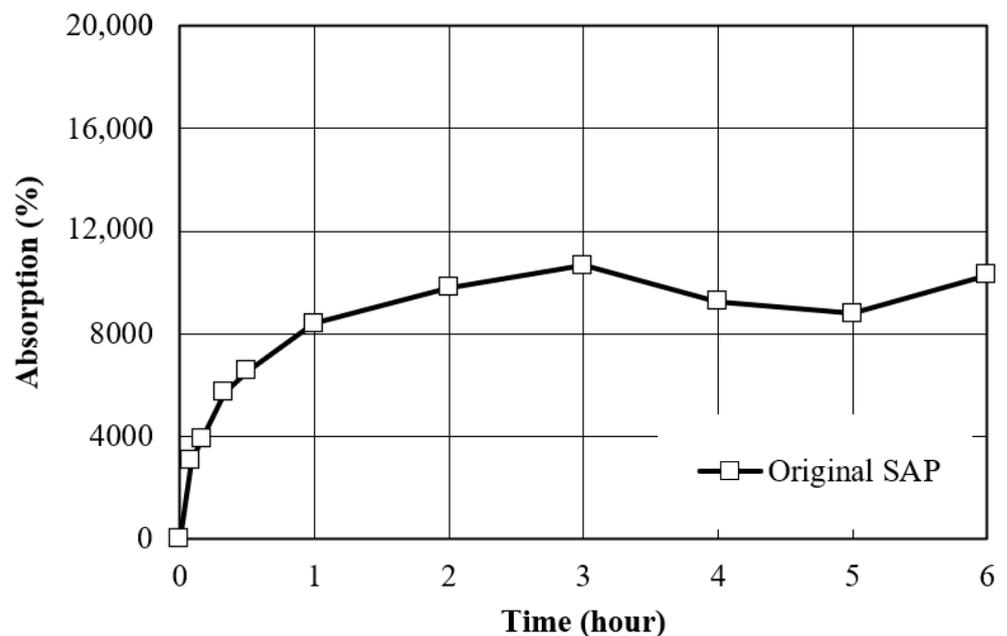
**Figure 4.** Absorption capacity of original dry SAP.
