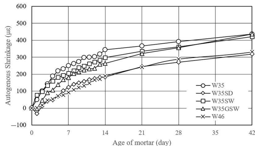
Figure 11. Autogenous shrinkage of mortar.
