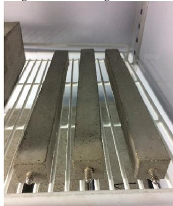
(b) Total shrinkage tested samples.
