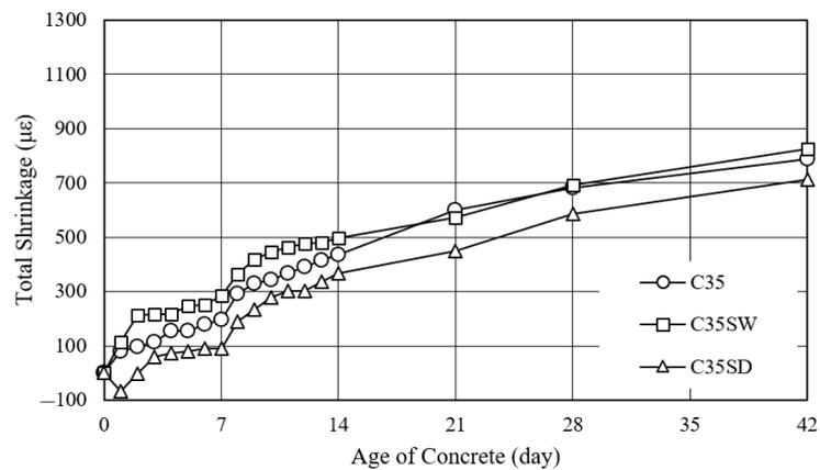
Figure 17. Total shrinkage of concrete.
