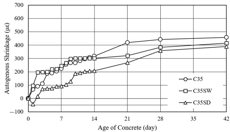
Figure 16. Autogenous shrinkage of concrete.
