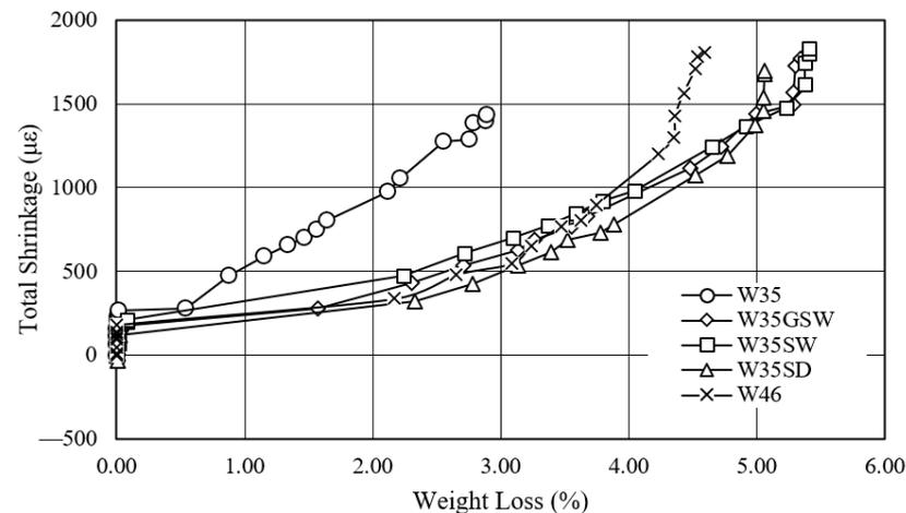
**Figure 15.** Relationship between the total shrinkage and weight loss of mortar.
