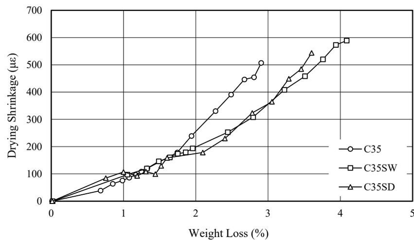
**Figure 19.** Relationship between the drying shrinkage and weight loss of concrete.
