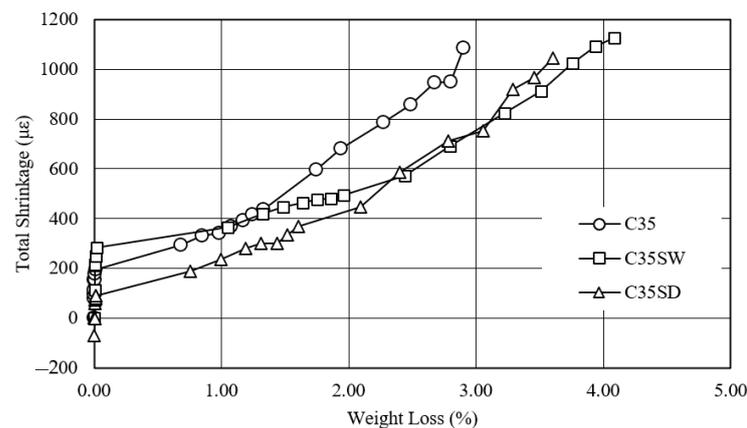
**Figure 20.** Relationship between the total shrinkage and weight loss of concrete.
