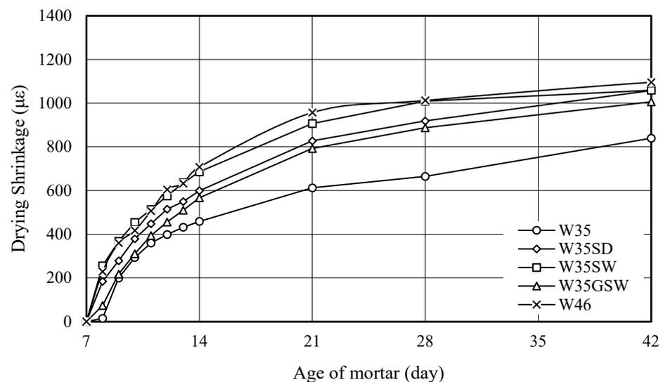
Figure 13. Drying shrinkage of mortar.
