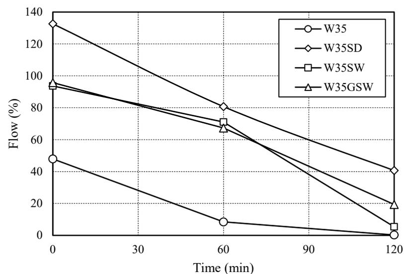
Figure 10. Flow rate of mortar.
