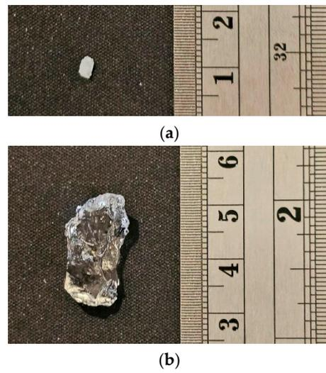
**Figure 1.** Particle size of SAP used in this study: (a) dry SAP; (b) wet SAP.
