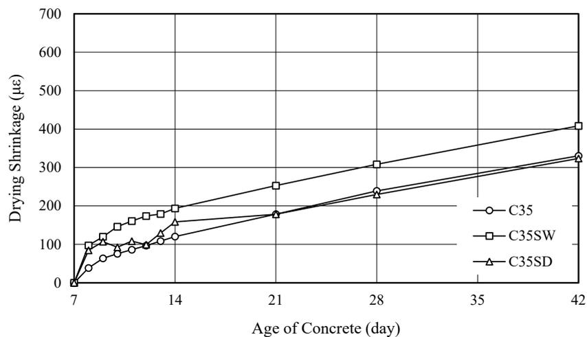
Figure 18. Drying shrinkage of concrete.
