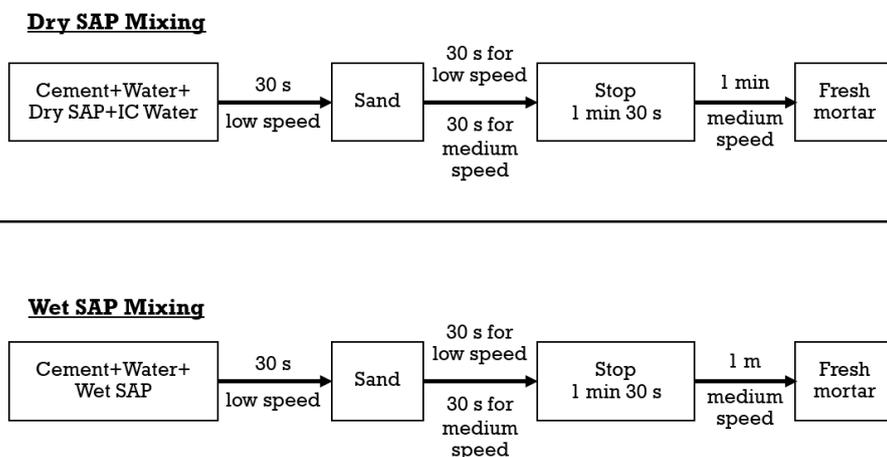
Figure 6. Mixing steps for mortar with SAP.
