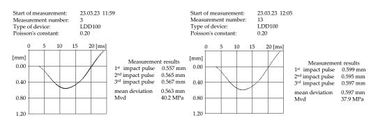
**Figure 8.** Immediate test results using LDD 100 on the surface of a 0/31.5 mm crushed aggregate layer and monitoring its dynamic response.
