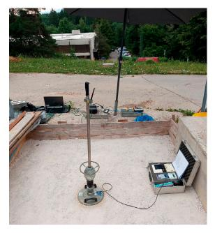
**Figure 7.** Implementation of dynamic load test using LDD 100 on the surface of crushed aggregate layer fr. 0/31.5 mm and monitoring of its dynamic response.
