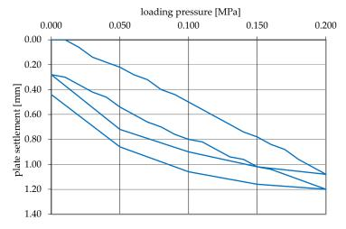
**Figure 6.** Output of the static test performed on the surface of the crushed aggregate layer of fr. 0/31.5 mm—plate settlement recorded at each change of 0.01 MPa in the loading pressure.
