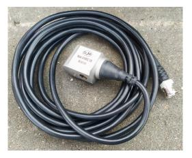
Figure 4. Single-axis accelerometer IEPE A/140/SC [25].
