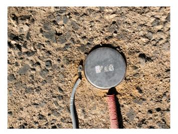
Figure 5. Mounting the sensors on the surface of foam glass aggregate.
