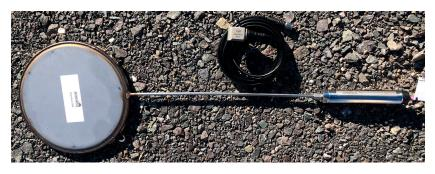
Figure 3. Pressure transducer Sisgeo L141 [24].
