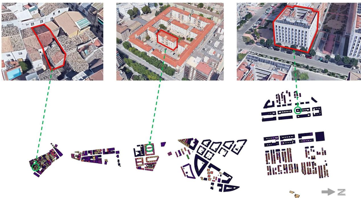
Figure 6. Selected benchmark buildings. Aerial view from Google Earth and location within the case study area in Jaén. Color ramp represents building’s heating demand per m<sup>2</sup>.
