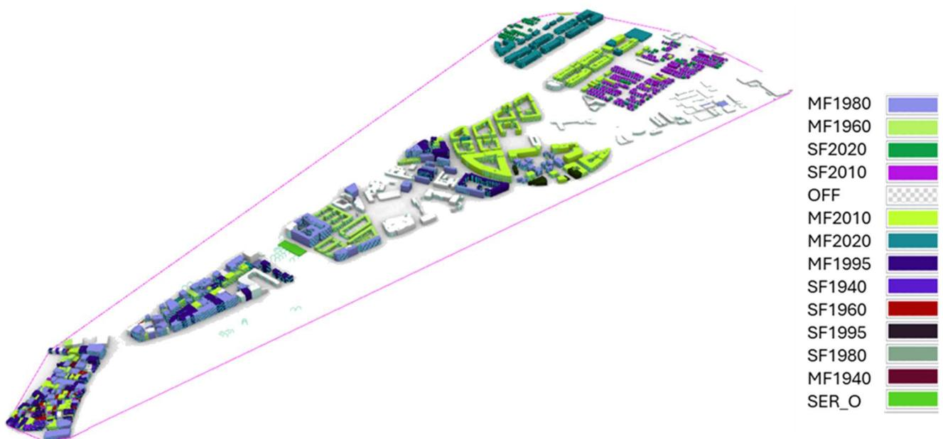
**Figure 2.** General overview of the UBEM model of the case study, modeled with UMI 3.0, Rhinoceros 6, and the UBEM.IO platform. The building typologies used are represented in color.
