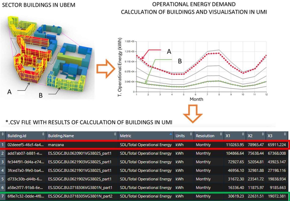
**Figure 4.** Sample output of results of buildings A and B from a UBEM model in UMI. Exploration of consumption results by different uses on a monthly basis. The results were imported in CSV format for processing and statistical analysis in R-Studio 2022.02.0. Note: \*.CSV is used to represent an undefined (\*) output file with ‘.csv’ extension.
