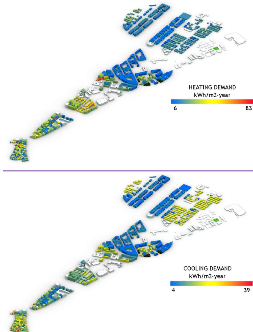
Figure 8. False color representation of heating and cooling demands normalized per square meter in the Jaén sector. Results from the GIS-UBEM obtained with the UMI.
