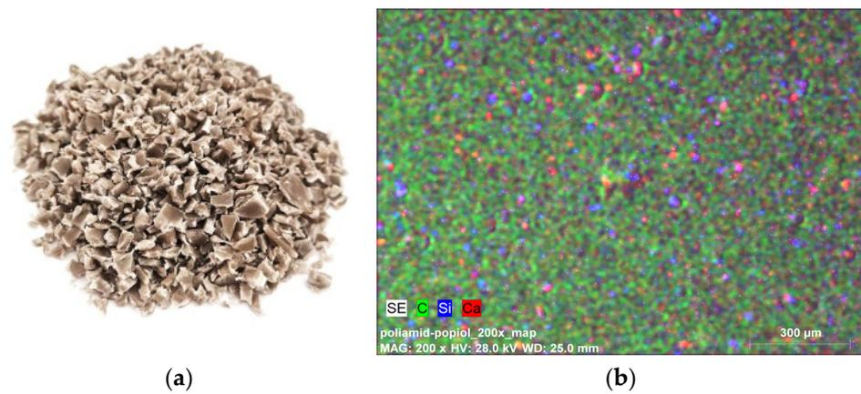
**Figure 1.** Waste polyamide 6 modified with 15% fly ash (a) and a microscope photo at 400× magnification with the dominant elements in this area (b).
