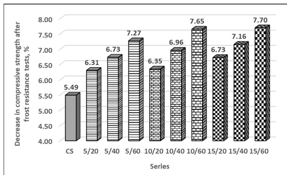
**Figure 6.** The compressive strength of investigated cement mortar after frost resistance tests.
