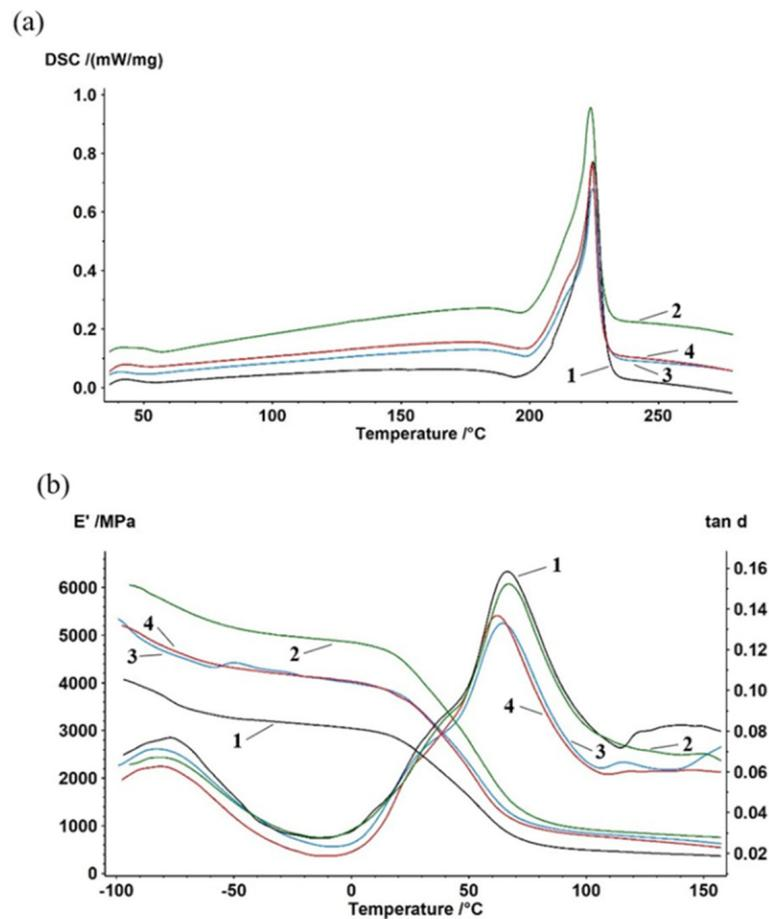
**Figure 2.** DSC (a) and DMTA (b) thermograms for fly ash-modified polyamide: 1—PA, 2—A + 5% biomass fly ash, 3—PA + 10% biomass fly ash, 4—PA + 15% biomass fly ash.
