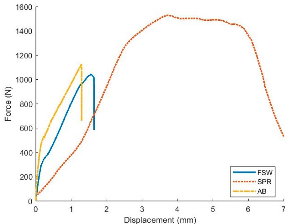
Figure 7. Force–displacement curves for the joining processes.
