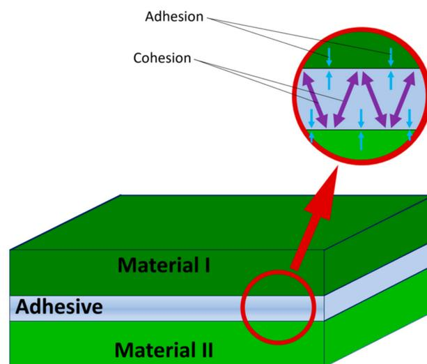
Figure 3. Adhesive bonding process [25].
