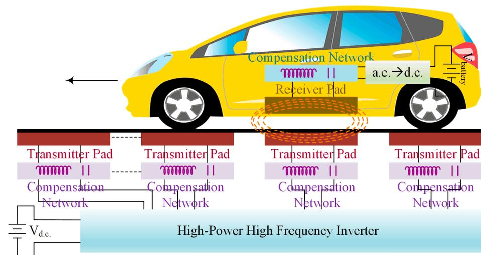
**Figure 2.** Representation of quasi-dynamic wireless charging system.
