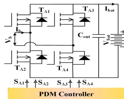
Figure 8. PDM-controlled active bridge rectifier.
