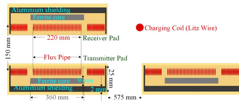
**Figure 4.** Geometry representation of quasi-dynamic charging coupler.
