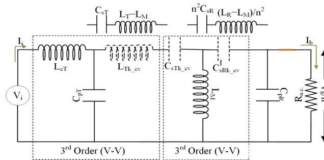
Figure 7. LCC-SP network’s a.c. equivalent circuit.
