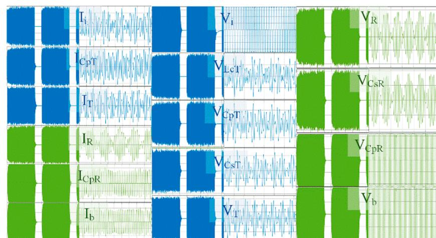
Figure 16. Simulation curves of LCC-SP network with 80% PDM.
