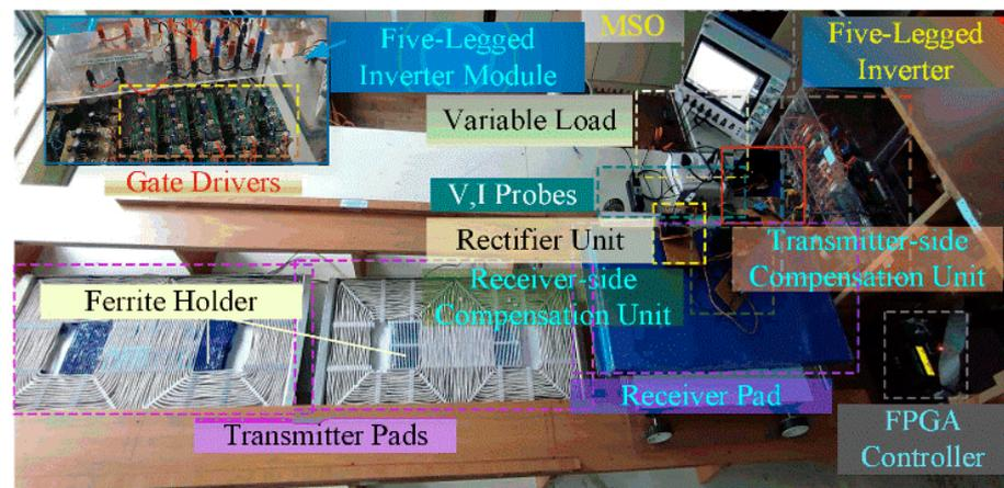
Figure 24. Experimental setup of the proposed charging system.
