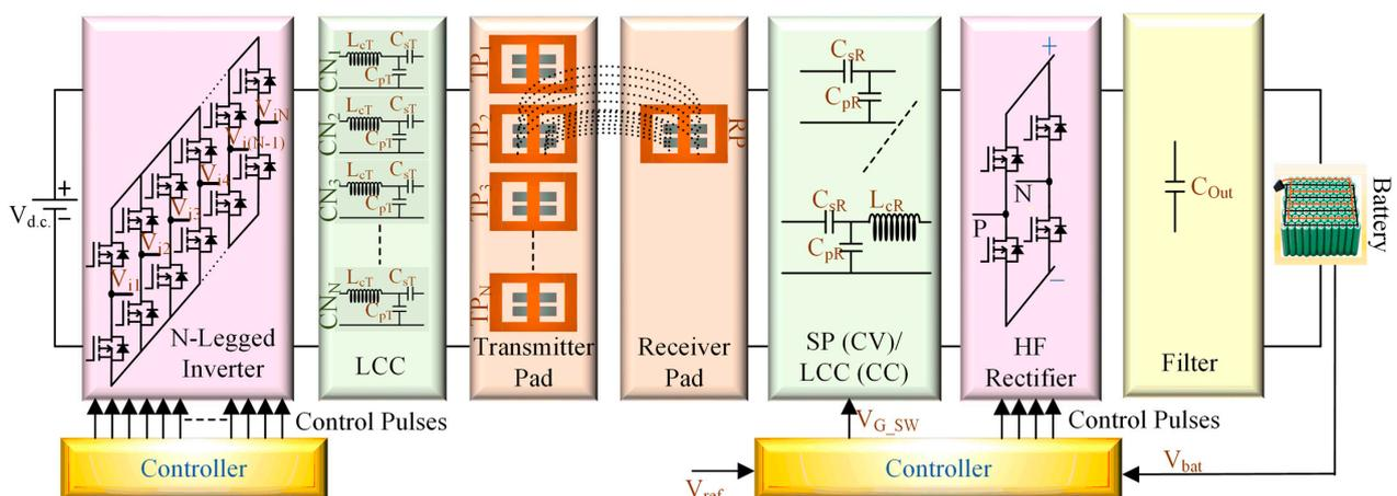
**Figure 3.** Block diagram of proposed quasi-dynamic wireless charging system.
