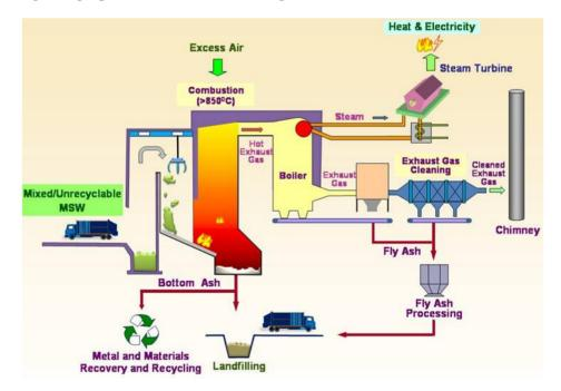
The MSW is fed into the furnace continually for incineration. Based on the Best Practical Means for the combustion of wastes, the combustion is enhanced by following the three T's guideline—high Temperature increases burnout, increased Turbulence exposes more waste surface and increases burnout, and a longer residence Time for the flue gas (>2 seconds) and the MSW increases
