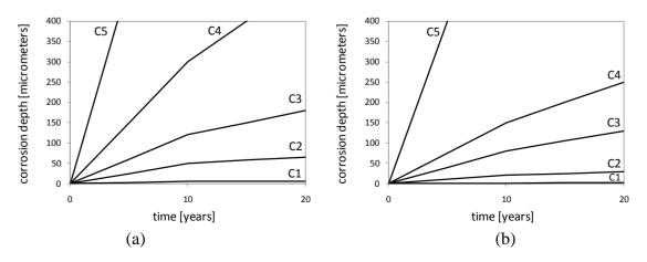
Some adjustment to these corrosion laws have been reported in Albrecht and Hall [22], where the authors proposed a new bi-linear model that accounts for a modified corrosion rate during the first year of exposure and a steady state during the subsequent years. An application of the modified bi-linear law for carbon and weathering steel for the upper and lower bound in the medium corrosivity category C3 is reported in Figure 3.
