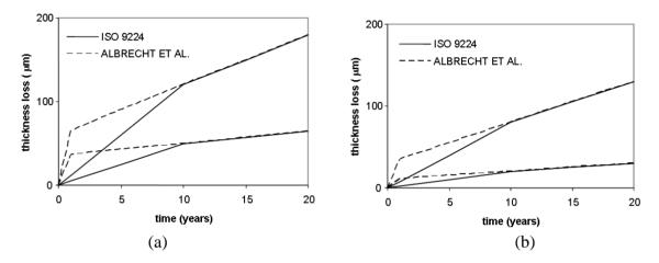
Recently, different models have been developed with the aim to generalize the corrosion loss over time for different environments, reporting the climate and pollutants variables as independent factors. In the following, two of these models are presented.
