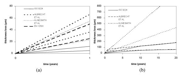
**Figure 5.** An application of the selected model to weathering for five years (a) and 20 years (b), corrosivity class C3.
