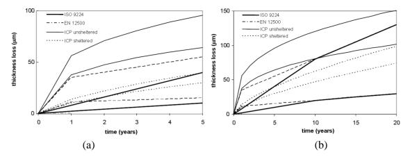
Indeed, as far as Klinesmith's corrosion model is concerned, the thickness loss values predicted for one year exposure are very close to EN 12500, but in the long-term, the models provides an average thickness loss of about 1.7 mm for a design life of 50 years, which is approximately 10-times more than the previsions given by the other models.
