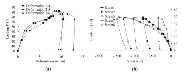
Figure 4. (a) Loading-Deformation Curve of W3. (b) Loading-Strain Curve of W2.
