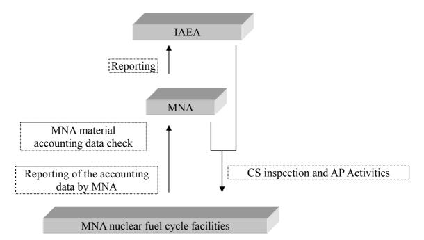
Figure 1. Inspection and material accounting system of a Multilateral Nuclear Approach (MNA).
