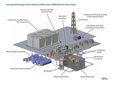
**Figure 5.** Layout of the GEN4 Energy plant. Source: [18].
