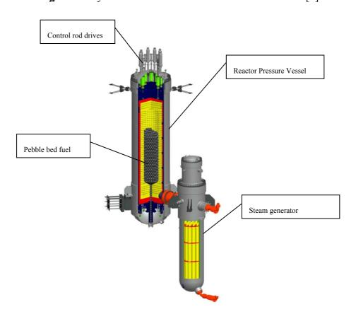
Figure 3. Layout of the HTR-PM reactor module. Source: [5].
