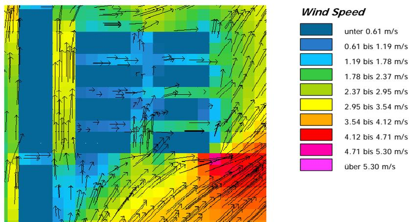
Proposal morphology helps SW wind to enter in the streets and ventilate the building's fachades and roofs. S-N ventilation in the central area transforms into transversal ventilation E-O in the adjacent area. Construction of taller barrers on the East side of the street could limit the wind use for all the right area of the city.
