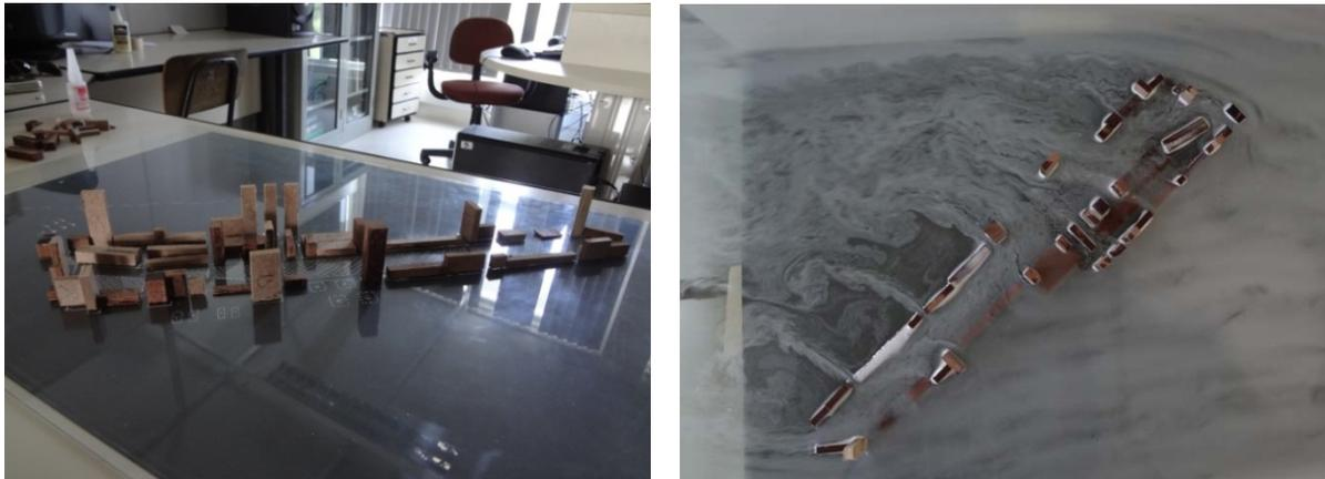
The most important results of the experiment are to show the transversal flows that could be blocked by dense construction in the east side of the street. The city sector behind the street needs the air flow to guarantee heat evacuation and air change possibility using natural ventilation design strategies.
