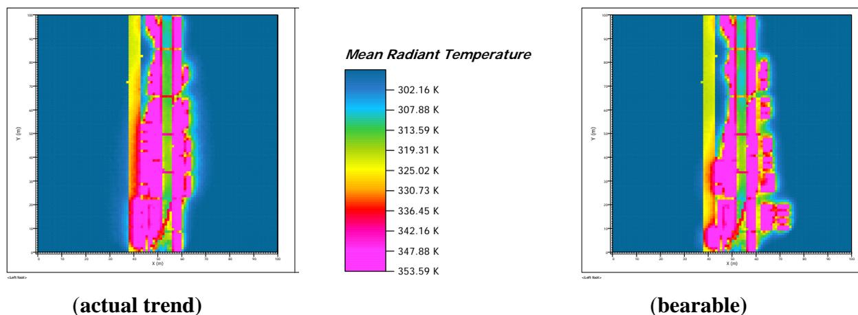
Results of more extensive simulations [23–25] show that uncontrolled development could cause an increase of about 0.5 °C in ambient temperature and up to 2 °C in mean radiant temperature, depending on the hours of exposition. In particular, the afternoon period is quite sensitive to different urban morphology near the site considered. Figure 8 shows the low radiation scenario at 15 h on a
