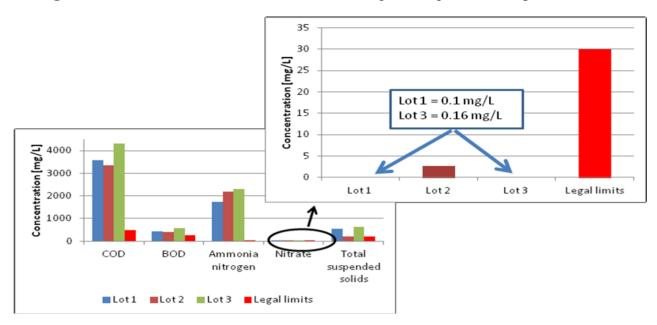
Figure 4. Initial concentrations of three leachate samples compared with regulation limits.
