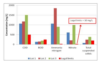
In none of the cases were the limits established for COD, ammonium and nitrate complied with. Furthermore, for the samples from Lots 2 and 3, the limits established for total suspended solids, total chromium, nickel and copper were not complied with, because of the mechanisms described above, which are only important on a laboratory scale, when stainless steel electrodes are used.
