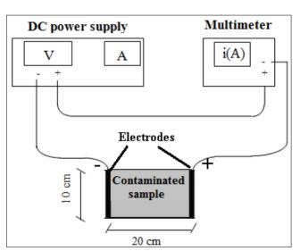
Figure 1. Experimental apparatus used in the tests.
